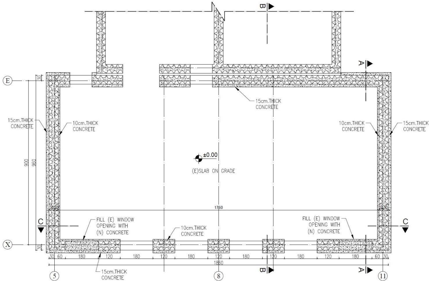
Figure B-12 Typology A typical gymnasium - ground floor plan.
