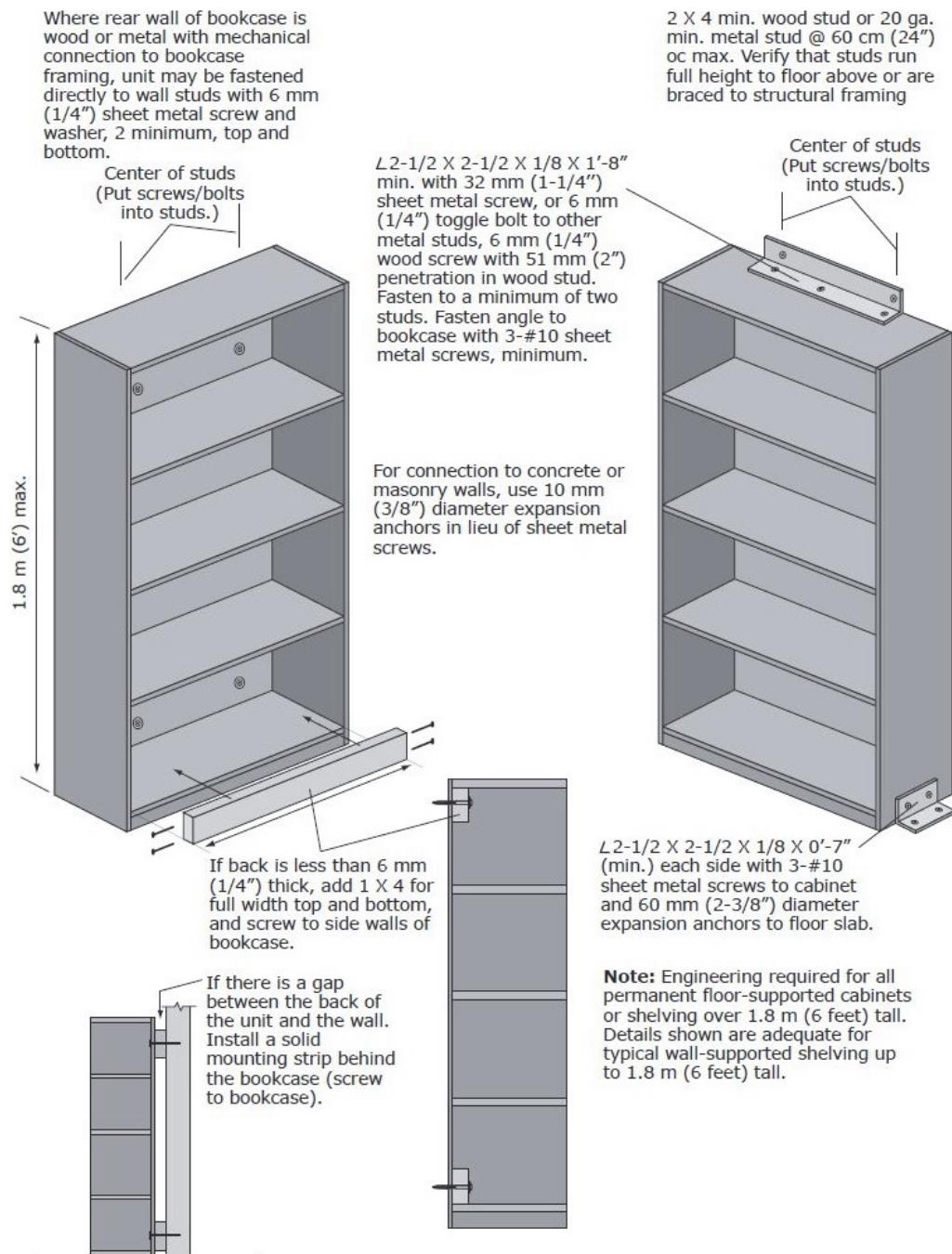
Figure 6-11 Example of bookshelf bracing and anchorage (adapted from FEMA, 2012).
