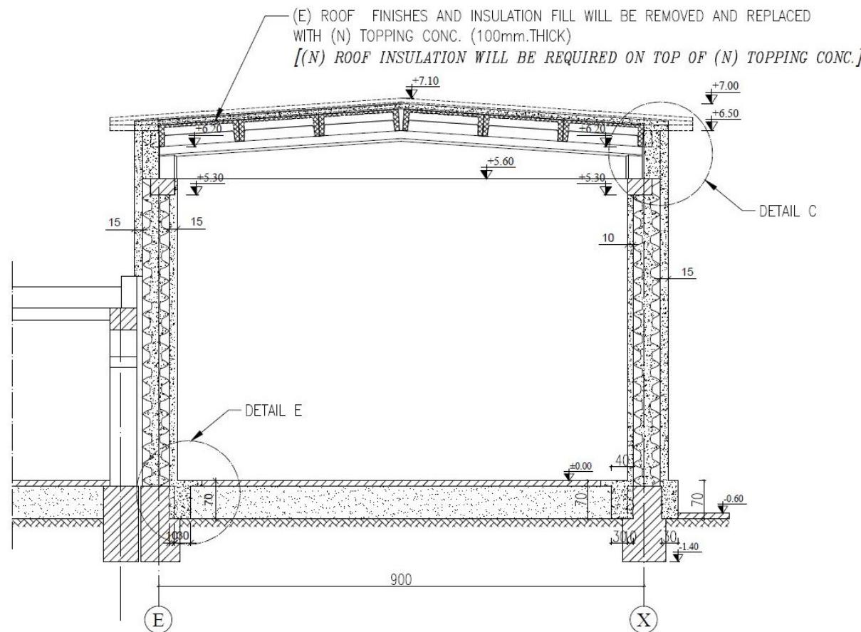
Figure B-15 Typology A typical gymnasium - transverse section.
