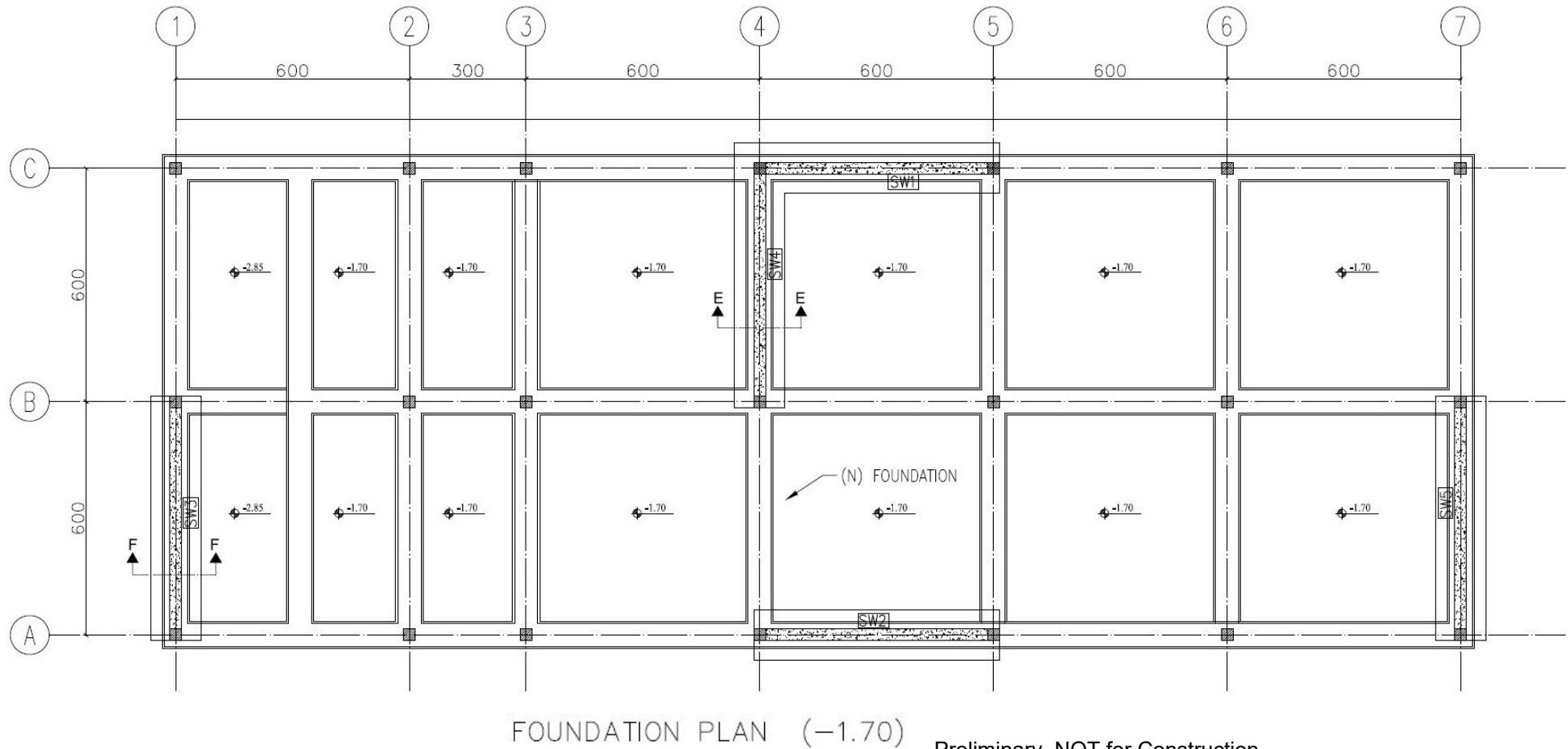
Figure C-1      Typology D-1 typical classroom - foundation plan.
