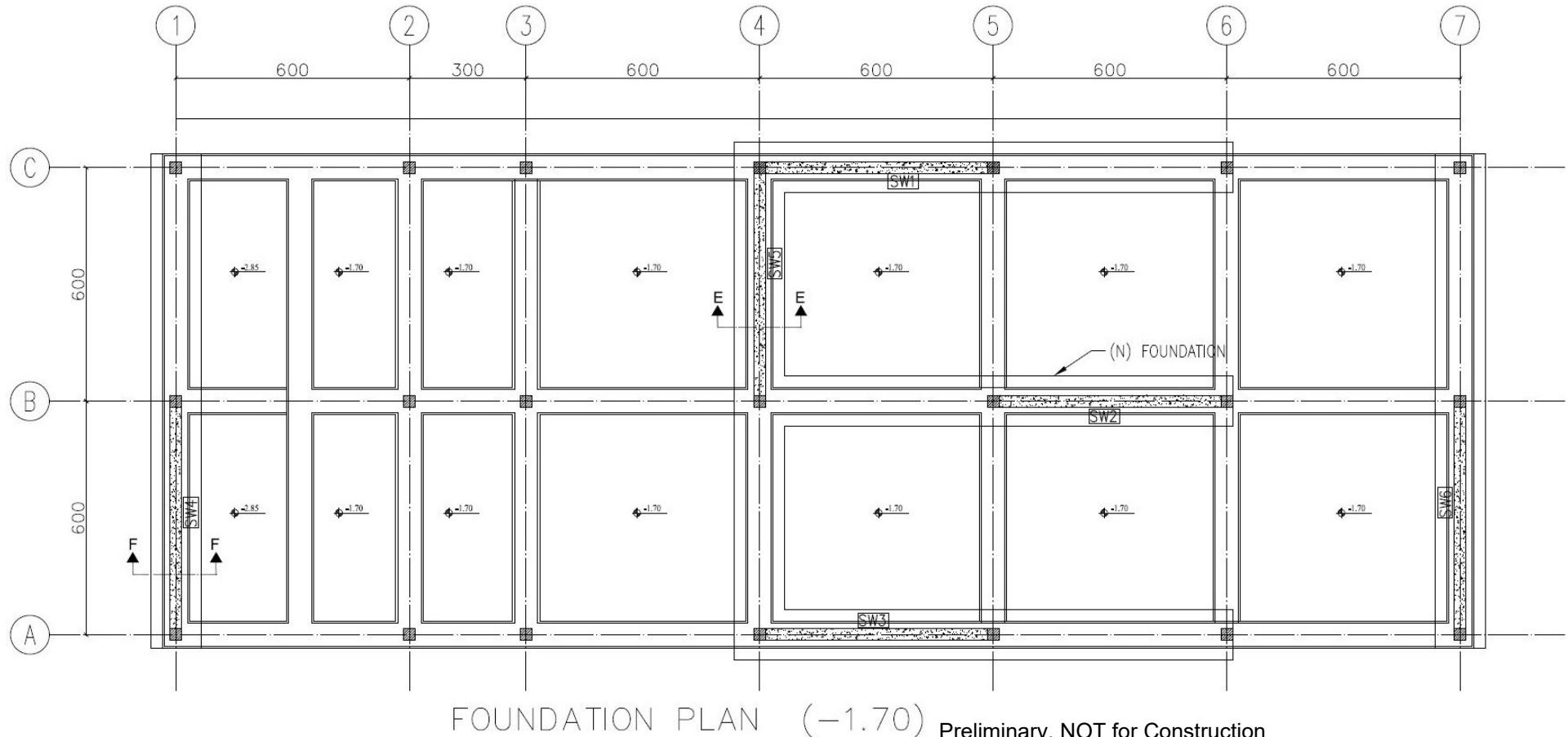
Figure D-1      Typology D-2 typical classroom - foundation plan.
