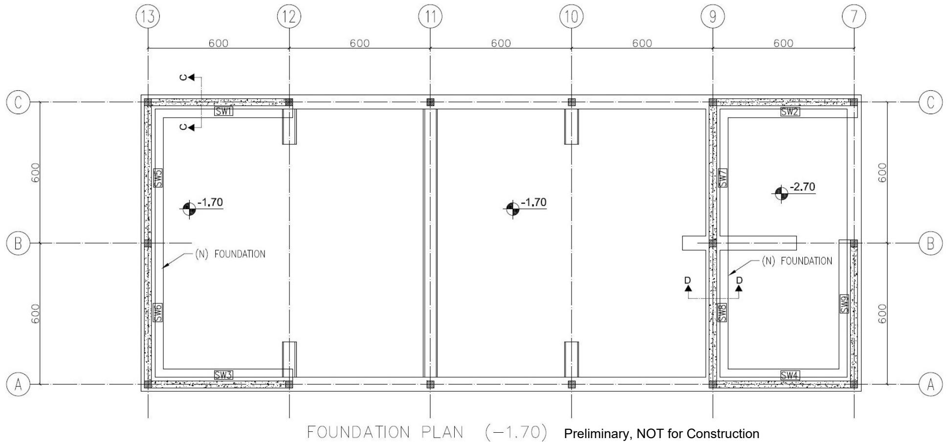
Figure C-6 Typology D-1 typical gymnasium - foundation plan.
