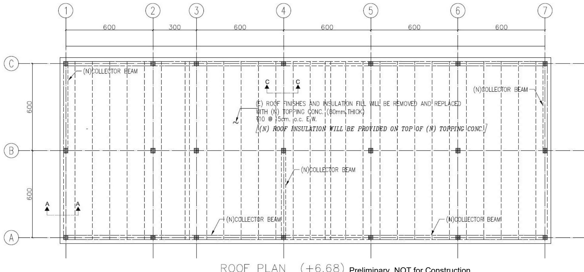
Figure C-4 Typology D-1 typical classroom - roof plan.
