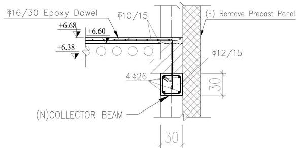
TYPICAL (N)COLLECTOR BEAM SECTION
