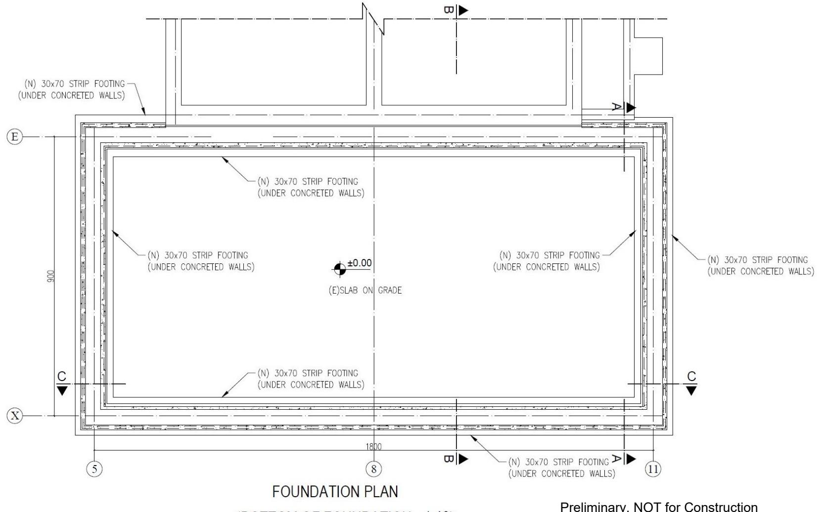
Figure B-11 Typology A typical gymnasium - foundation plan.
