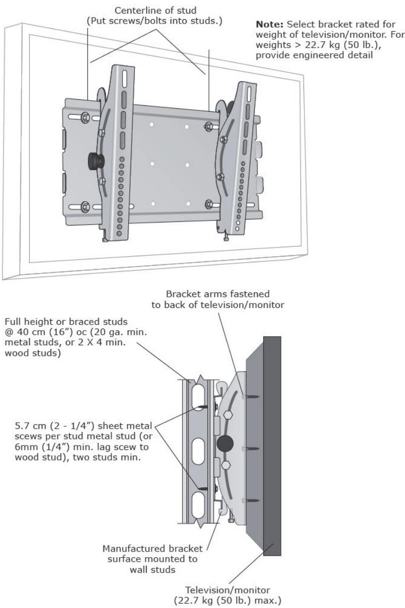
Figure 6-10 Example of earthquake mounting bracket for television monitors
