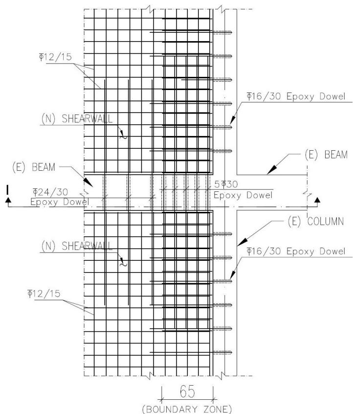
TYPICAL BOUNDARY ZONE & WEB REINFORCEMENT CONTINUITY DETAIL
