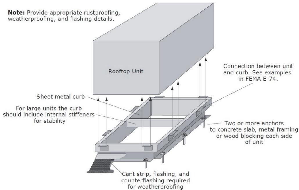
Figure 6-5 Example detail for roof-mounted HVAC unit (FEMA, 2012).
