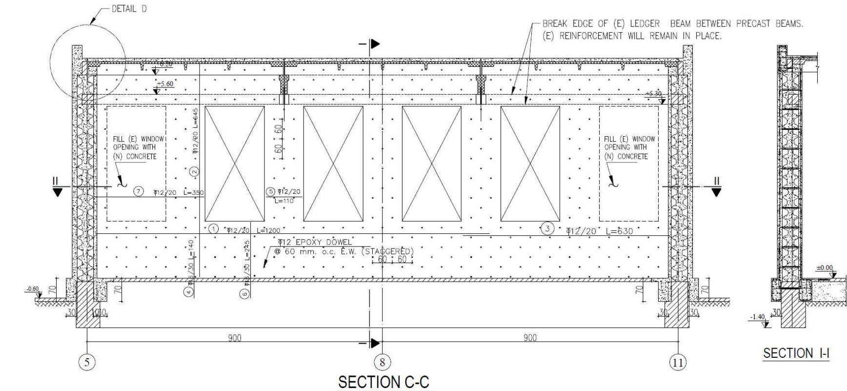
Figure B-16 Typology A typical gymnasium - longitudinal section and details.
