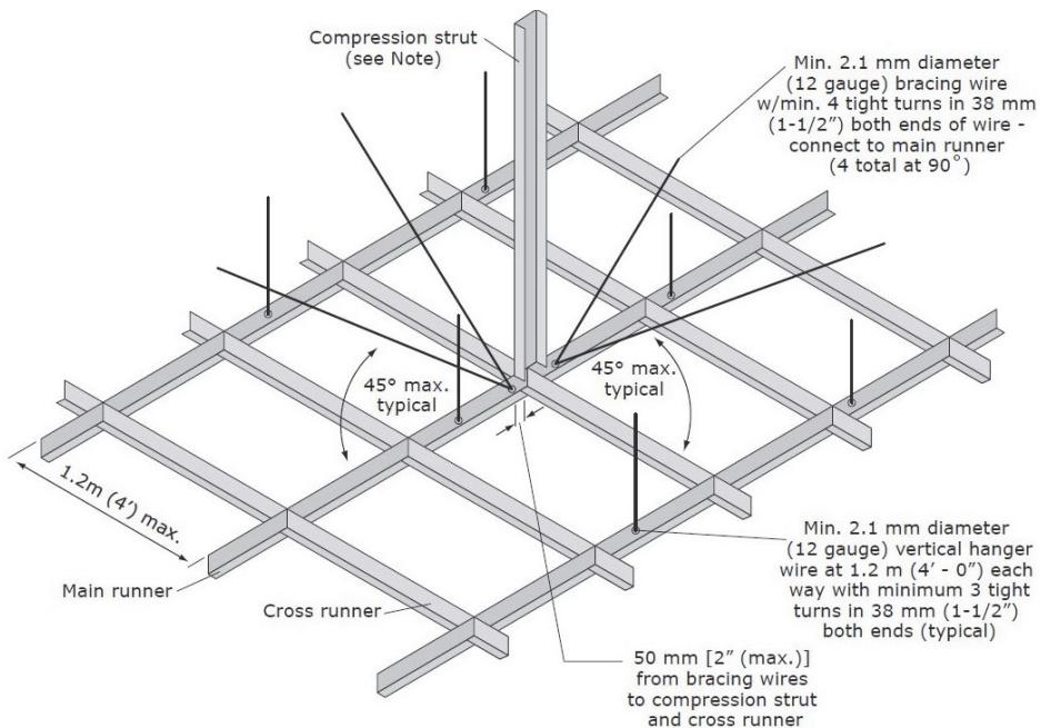
Figure 6-1 Example of bracing for suspended ceilings (adapted from FEMA, 2012).
