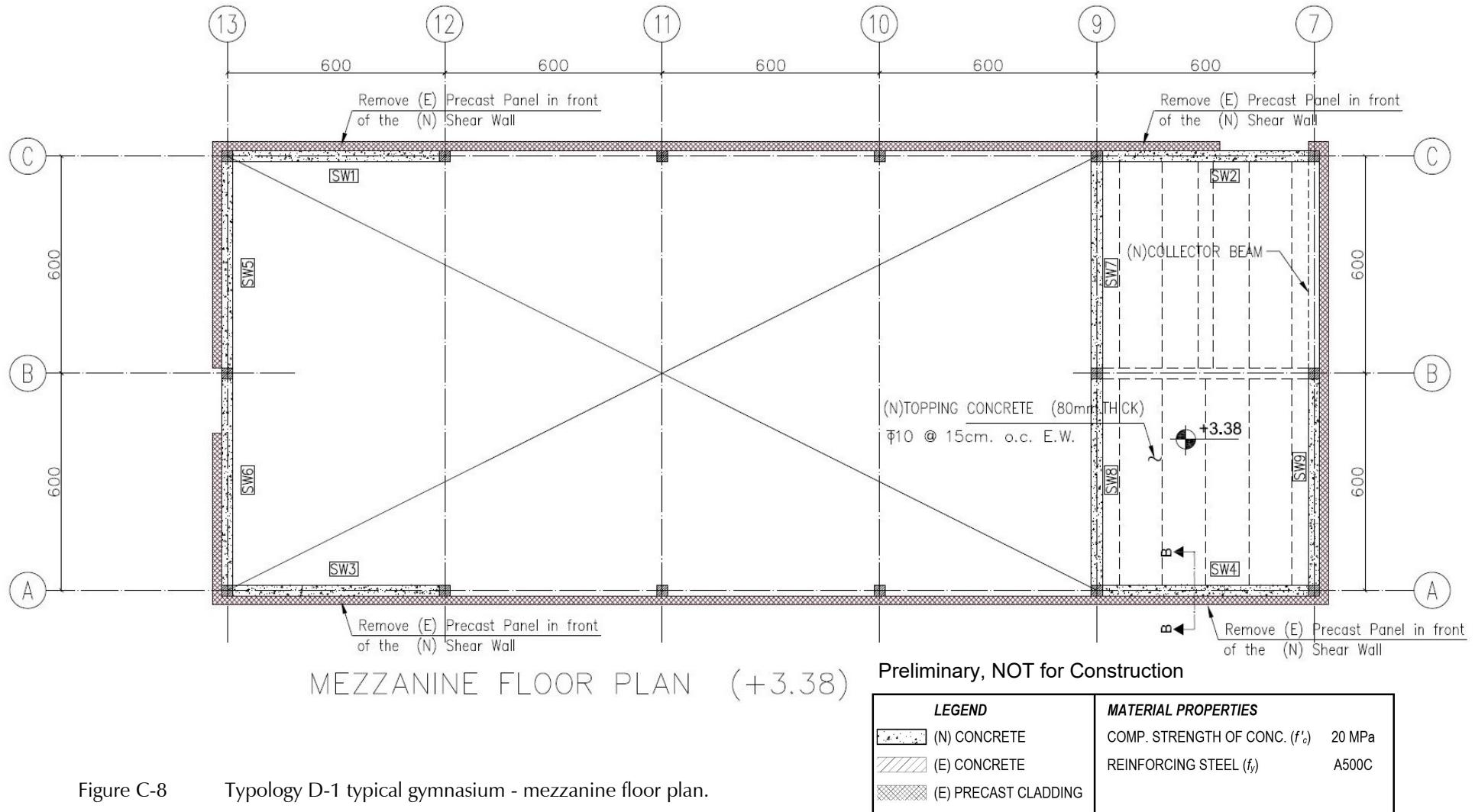
Figure C-8 Typology D-1 typical gymnasium - mezzanine floor plan.
