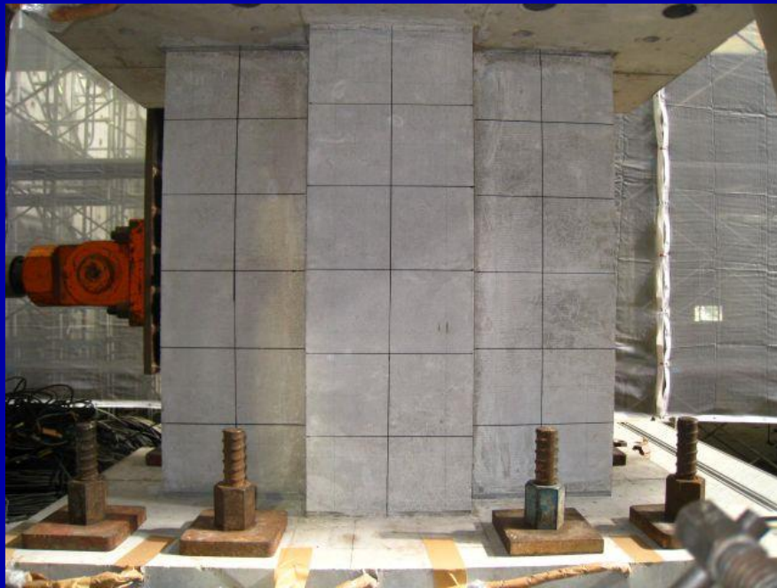
A column with side-walls
