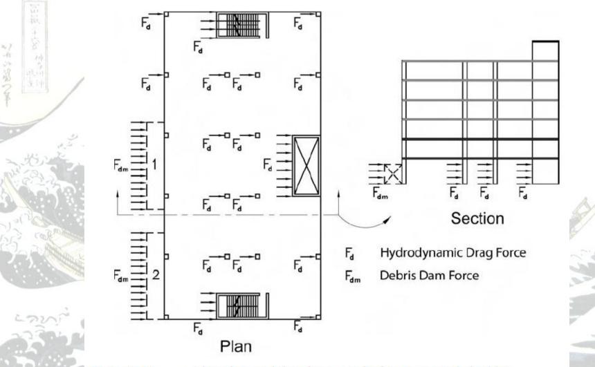
Figure 6-11 Debris dam and drag forces applied to an example building
