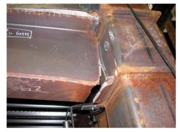
Fracture at beam-ends (E-defense experiment)
