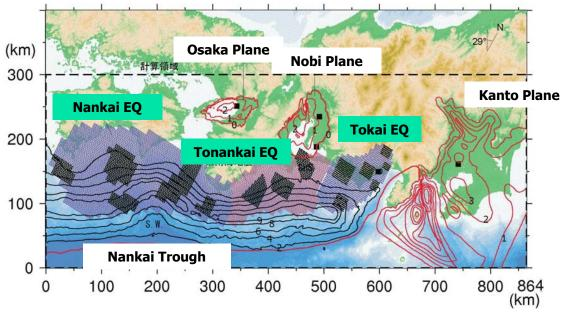
Earthquake Source Model for Expected Tokai, Tonankai and Nankai Earthquakes
