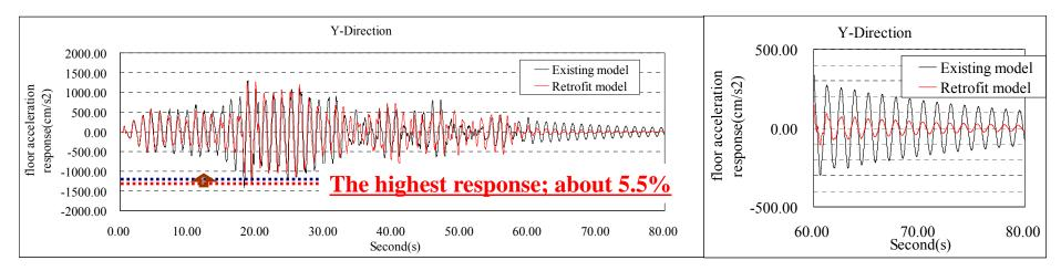
Fig. Time History of Response acceleration (Y-direction / L20)
