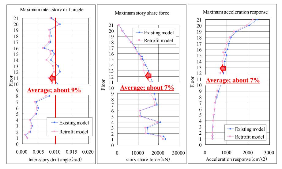
Fig. Maximum Response of Y-direction
