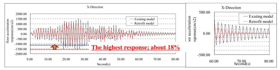
Fig. Time History of Response acceleration (X-direction / L20)
