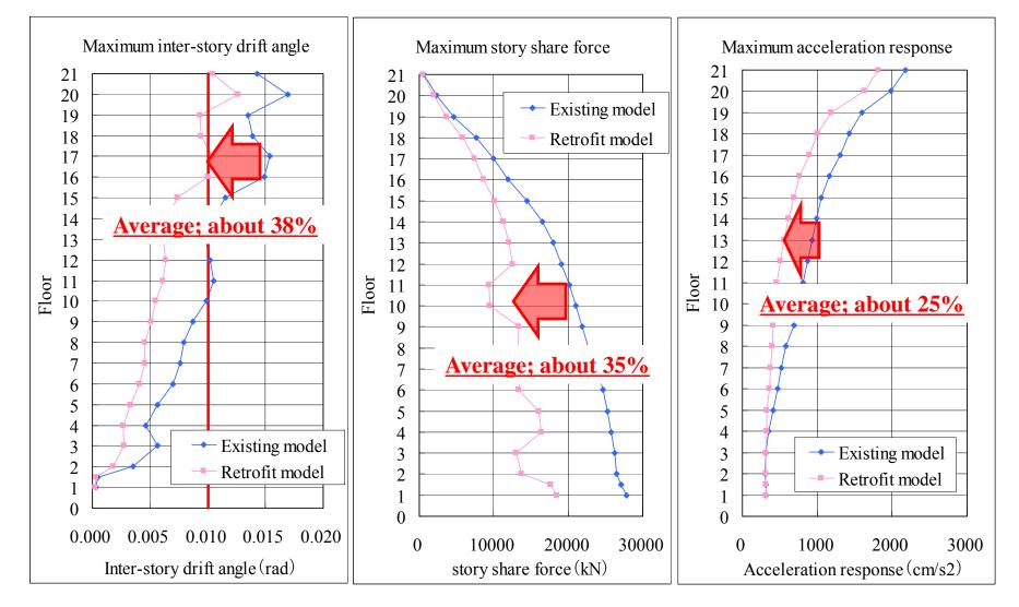
Fig. Maximum Response of X-direction
