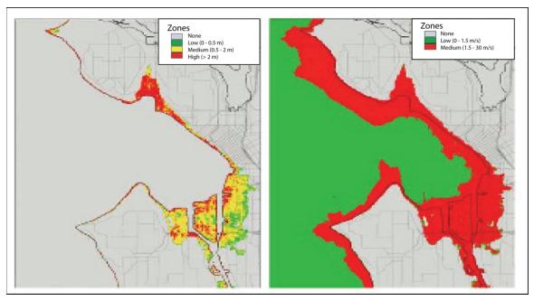
Figure 3-2 Tsunami inundation modeling products for Seattle, Washington. Left panel: zoned estimates of maximum inundation depth.
