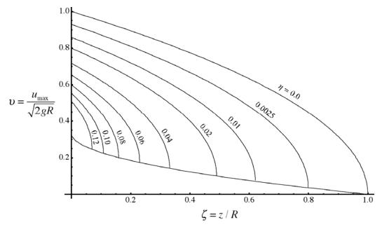
Figure E-1 Maximum flow velocity of depth, *d*, at the ground elevation, *z*, and maximum runup elevation, *R*. The bottom curve represents the lower limit of maximum flow velocity.
