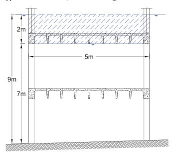
Figure C-2 Condition resulting in buoyant forces.
