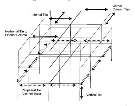
Note: The required Exterior Column, Exterior Wall, and Corner Column Tie forces may be provided partly or wholly by the same reinforcement that is used to meet the Peripheral Tie requirement.
