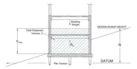
Figure 6-5 Buoyant forces on an overall building with watertight lower levels.
