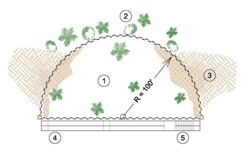
Figure B-5 Example escape berm plan layout.
