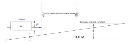
Figure 6-8 Waterborne debris impact force.
