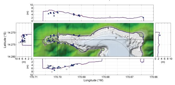
Figure 6-3 Comparison between numerical modeling (blue line) and field measurement of run-up (white dots) and flow elevations (blue dots) at Pago Pago Harbor, American Samoa (Yamazaki et al. 2011).
