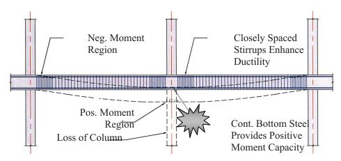
Figure 6-15 Detailing of reinforcing steel for potential loss of a supporting column.
