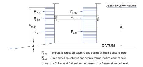
Figure 6-7 Hydrodynamic impulsive and drag forces on components of a building subjected to inundation by a tsunami bore.
