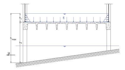
Figure 6-11 Gravity loads exerted on an elevated floor with water retained by exterior walls during rapid drawdown.
