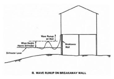
Figure 7-1 Effect of breakaway walls on waves (FEMA, 2005).
