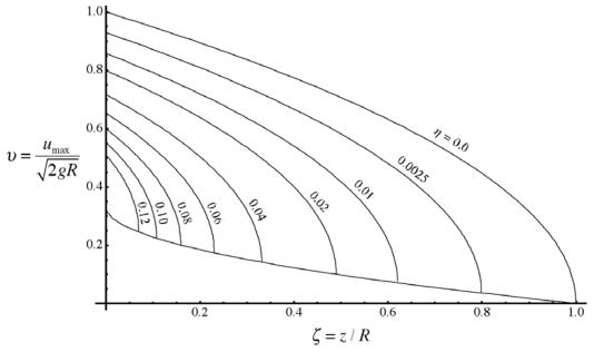
Figure 6-9 Maximum flow velocity of depth, *d*, at the ground elevation, *z*, and maximum runup elevation, *R*. The bottom curve represents the lower limit of maximum flow velocity.
