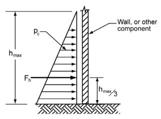
Figure 6-4 Hydrostatic force distribution and location of resultant.
