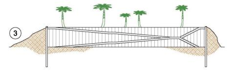
Figure B-7 Example escape berm rear elevation.
