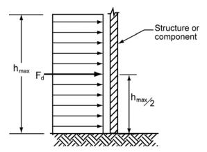
Figure 6-6 Hydrodynamic force distribution and location of resultant.
