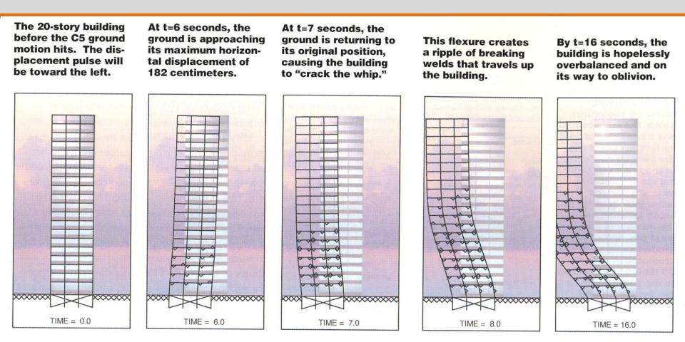
triangles indicate failure of welded beam-column connections
