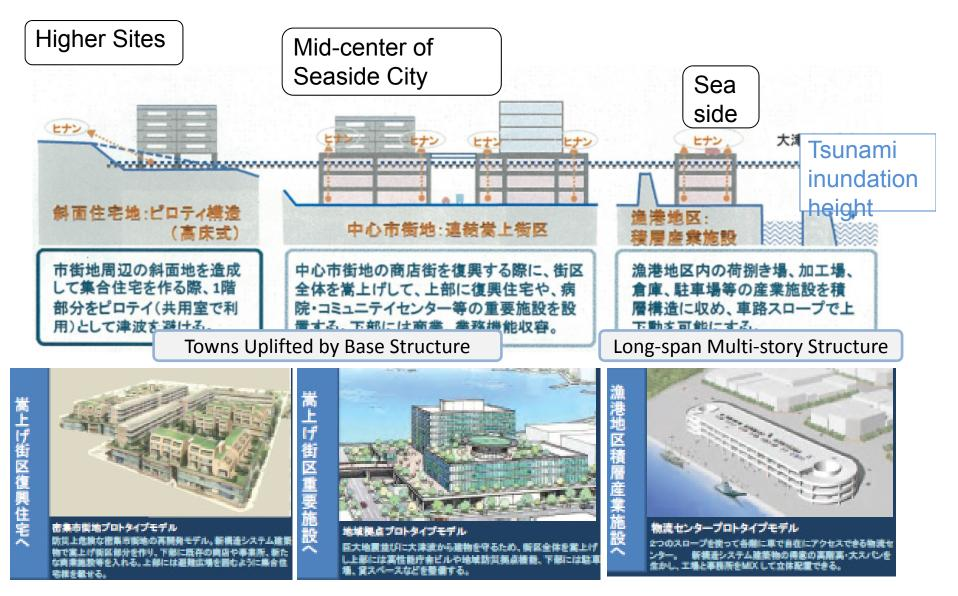
Concept of Proposed Re-constructed City with New Structure System Buildings
