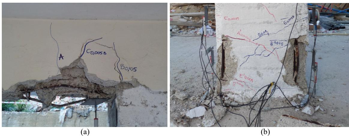
Figure 7. The damage seen in (a) K12 beam at 0.75 % drift ratio and (b) S14 column at 1.50% drift ratio.
