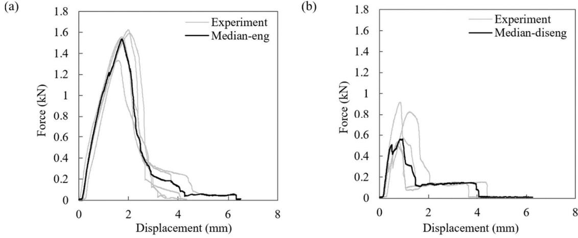
Figure 5. Results of tensile tests on CT-MT joints without seismic clips with
