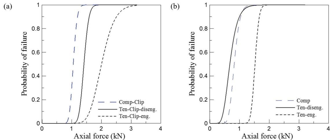
Figure 10. Fragility curves for all CT-MT joint tests (a) with, and (b) without seismic clip.
