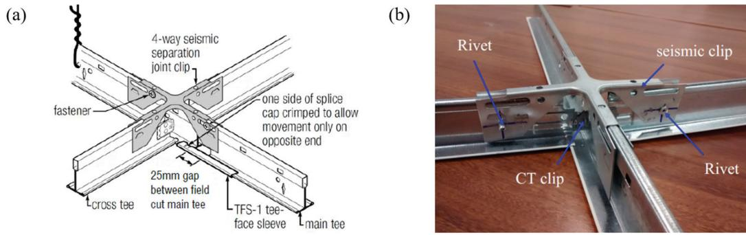
Figure 1. (a) DH4 seismic clip as seismic joint; (b) CT-MT connection specimen with seismic clip and 2 rivets on CTs.
