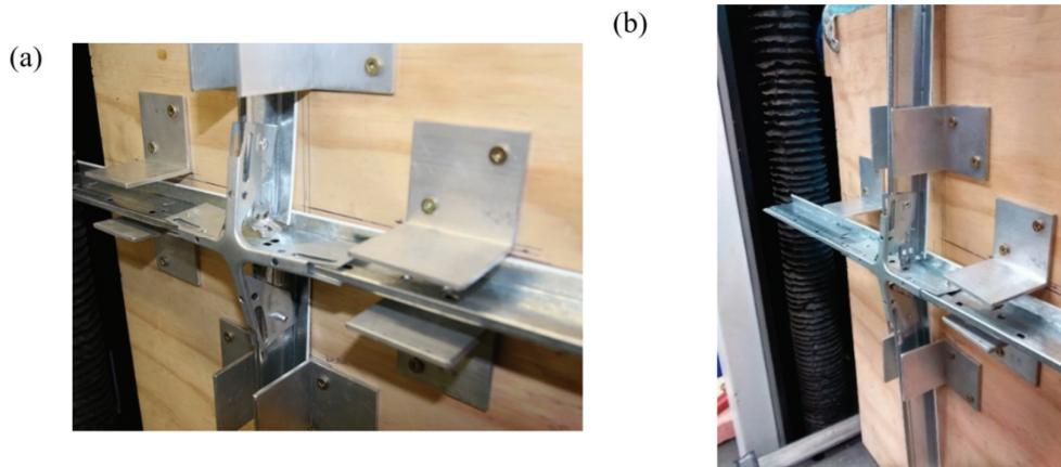
Figure 8. Failure in CT-MT joints with seismic clip: (a) bending in CT clip, and (b) out of plane buckling
