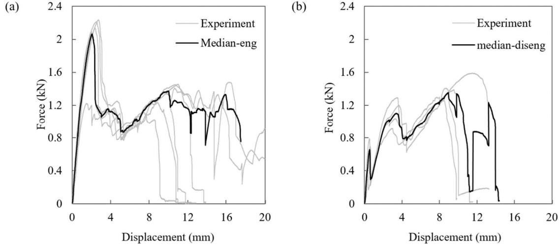
Figure 6. Results of tensile tests on CT-MT joints with seismic clips with
