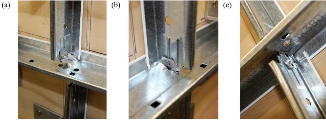
Figure 7. Failure of CT-MT joint in compression.
