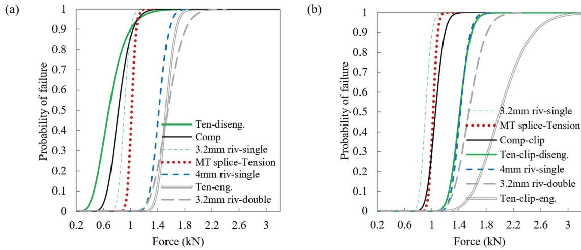
Figure 11. Fragility curves comparing other ceiling components (Paganotti 2010, Pourali et al. 2016) with CT-MT connections (a) without, and (b) with seismic clips.
