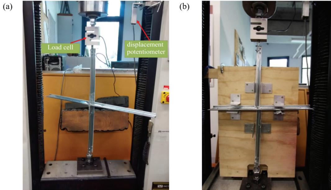
Figure 2. Test setup in (a) tension, and (b) compression tests
