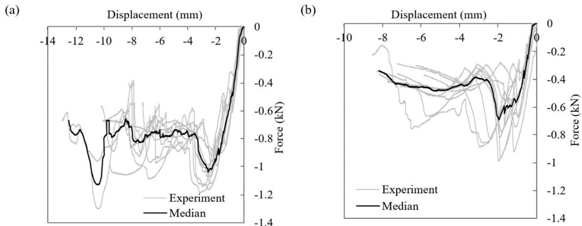
Figure 9. Results of compression tests on CT-MT joints (a) with, and (b) without seismic clips.
