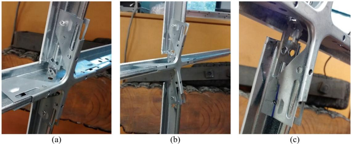
Figure 4. Failure of CT-MT joint with seismic clip in tension.
