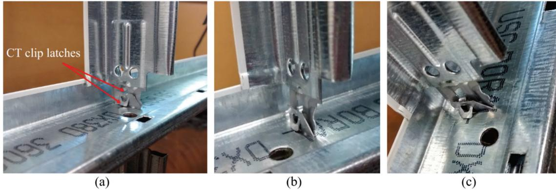
Figure 3. Mechanism of failure due to yielding in CT clip with the clip well engaged.
