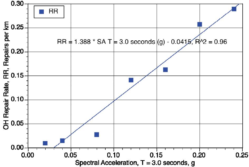
Figure 3. Repair rate, overheads, using PSA ( $T = 3.0$  seconds).
