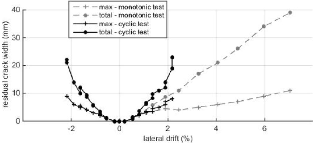
Figure 5. Residual crack widths (maximum and total) for specimen Cyc (black) and Mono (grey).
