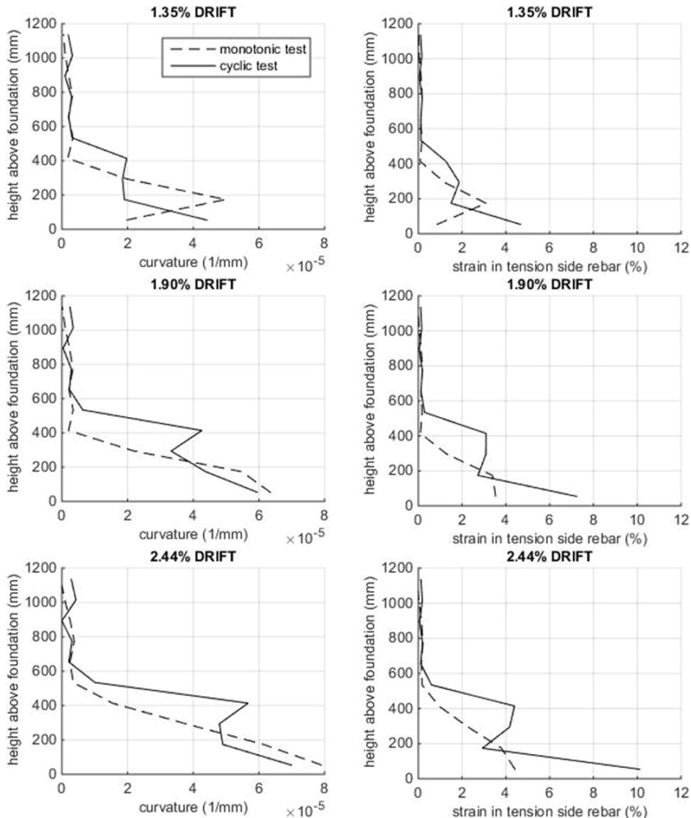
Figure 7. Distribution of curvatures and strains in tension side reinforcement at increasing drift levels for specimen Cyc (solid line) and Mono (dashed line).
