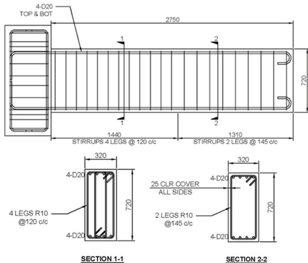
*Figure 3. Specimen detailing*
