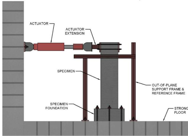
*Figure 2. Rendering of test set-up*
