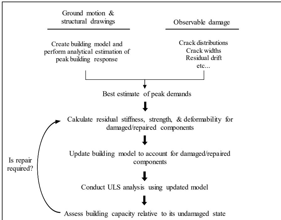
Figure 1. Flowchart of proposed post-earthquake assessment methodology.
