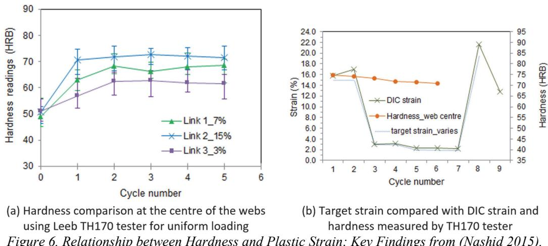
(a) Hardness comparison at the centre of the webs using Leeb TH170 tester for uniform loading
