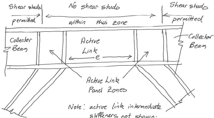
Figure 4. Terminology for EBF active link components.
