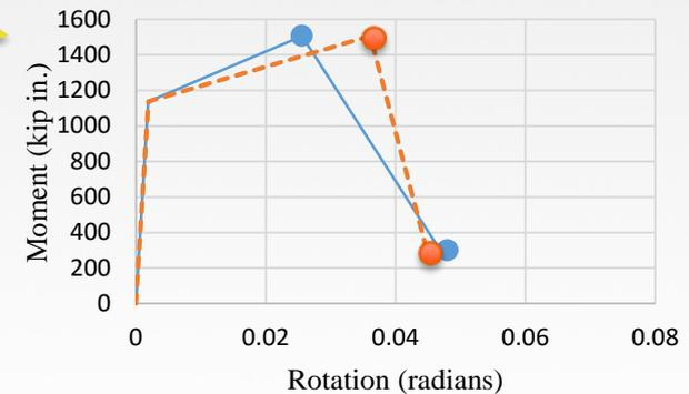
— ASCE 41-13 beam    - - - New beam model
