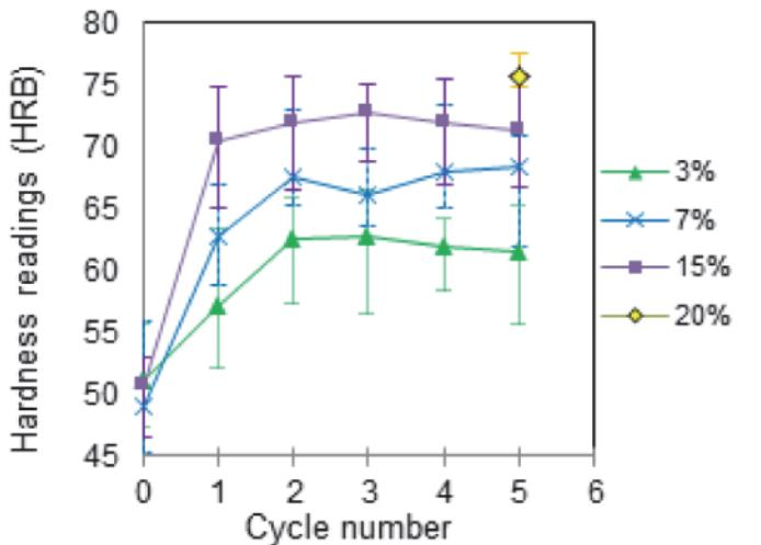
Fig. 5.4 Hardness distribution against cyclic number
