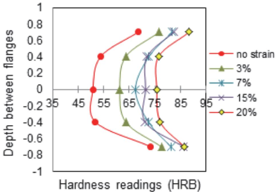
Hardness from different plastic strain at normalized link depths
