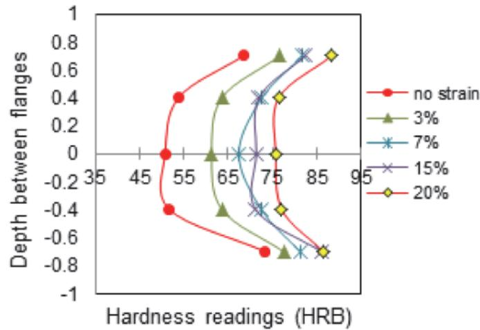
Fig. 5.3 Hardness from different plastic strain at normalized link depths
