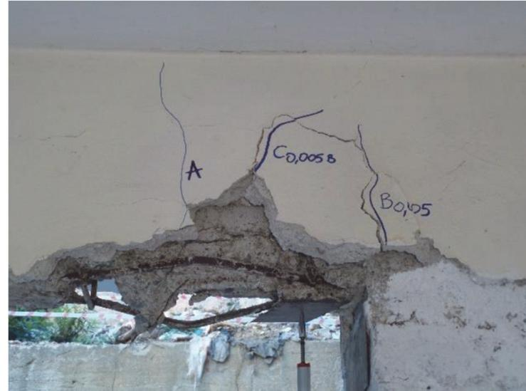
The beam compression bars buckled at 0.75 % drift ratio
