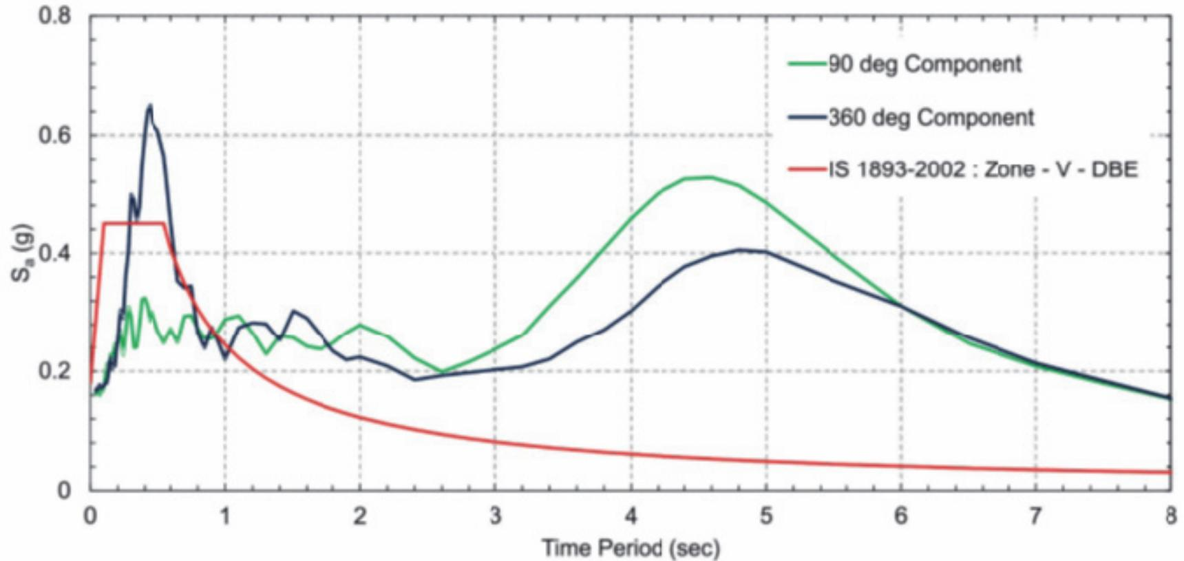
The shakings were larger than the design level for all structures except very stiff ( $T < 0.3s$ ) structures; i.e. 1-2 storey stiff load bearing houses, Rana era palaces with thick stiff walls
