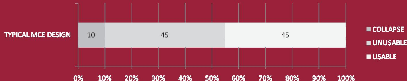
*Design code's assigned probability of collapse, major damage rendering a building unusable, and minor damage permitting building usage (ASCE 7-10, ATC 63)*
