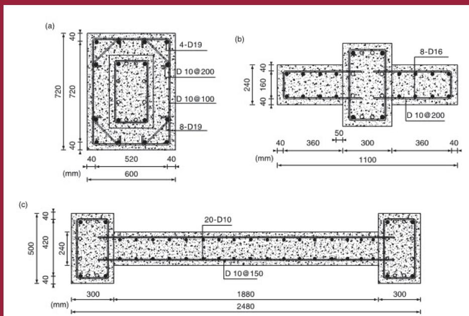
Typical Reinforcing Cross Sections: (a) Existing Column Jacketing; (b) Shear Panels Adjacent to Existing Columns; Shear Wall Between Existing Columns (Hsiao et al. 2014)
