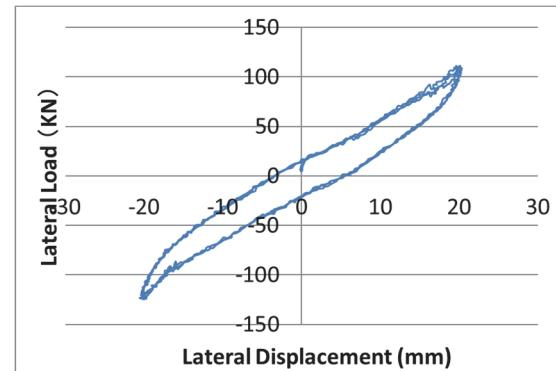
*Figure 9. Lateral loading test for rubber bearings*
