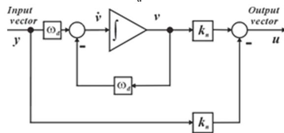
Figure 7. Block diagram of the oil dampers
