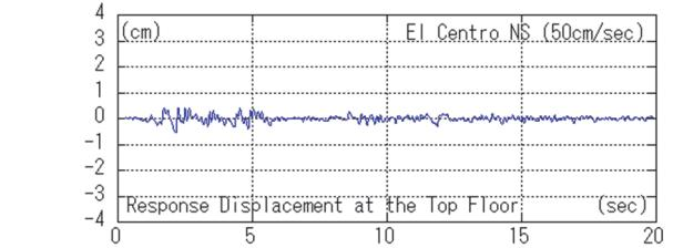
*Figure 13. With damper coefficient of 100KNsec/mm*
