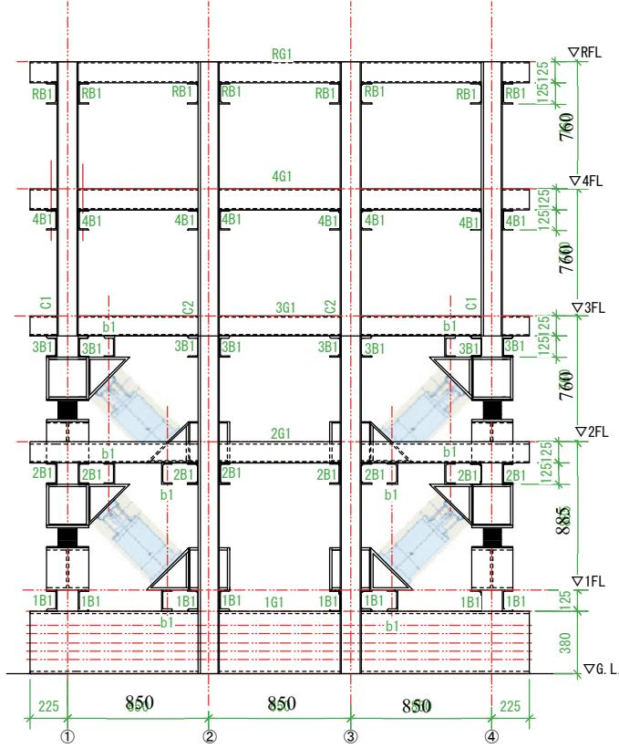
*Figure 2. The Axis-A of the specimen frame*
