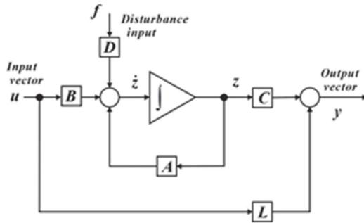
Figure 5. Block diagram of the frame dynamics without dampers
