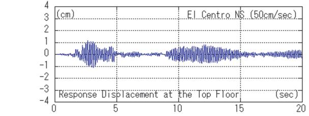
*Figure 12. With damper coefficient 0.50KNsec/mm*
