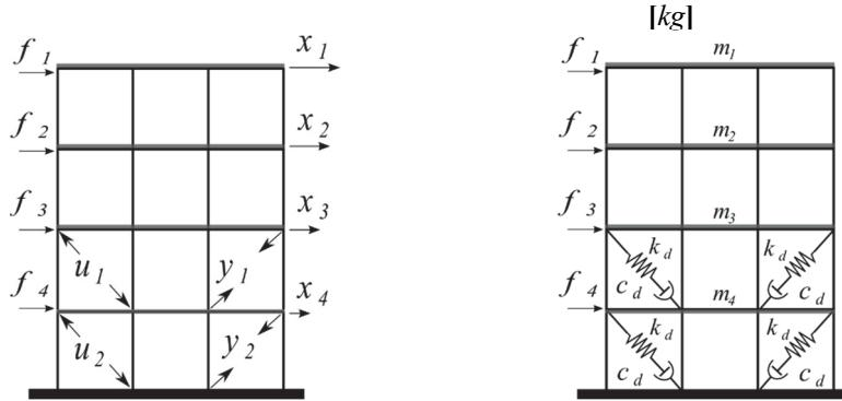
Figure 4. Interaction between Frame Deformation and Damper Reaction
