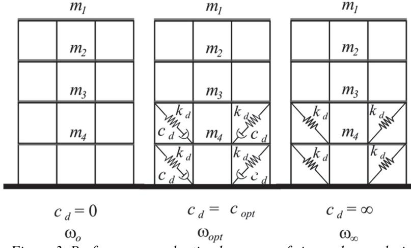
Figure 3. Performance evaluation by means of eigenvalue analysis
