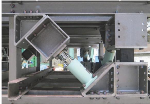
*Photo 1. Installation of oil damper and laminated rubber bearing*
