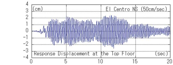
*Figure 11. With damper coefficient 0.01KNsec/mm*
