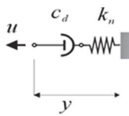
Figure 6. The oil damper model
