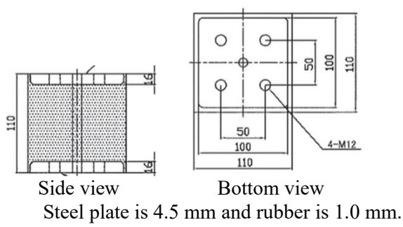
*Figure 8. The laminated rubber bearing*
