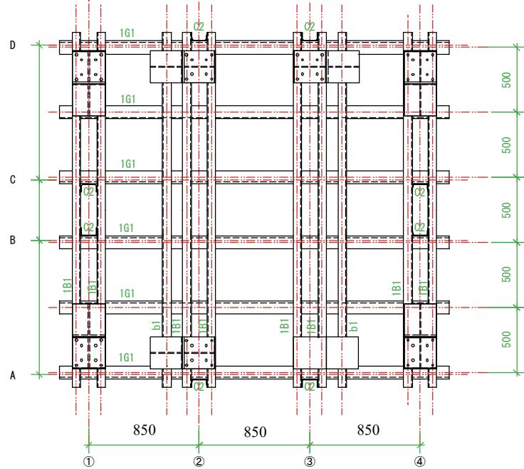
*Figure 1. The ground floor plan of the specimen frame*
