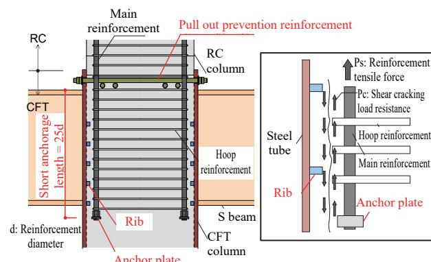
Figure 8. Detail of the structural connection method
