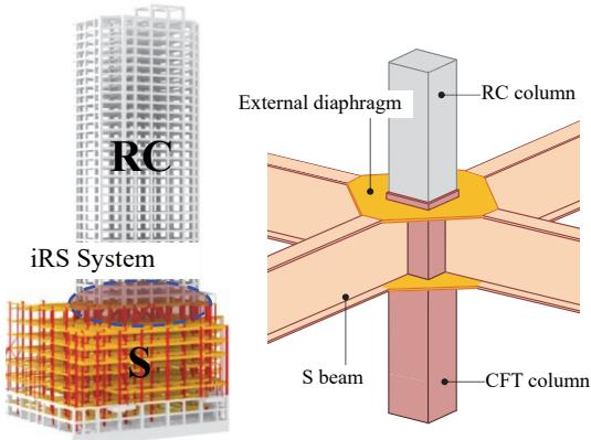
Figure 7. Structural method for connecting RC columns and CFT columns
