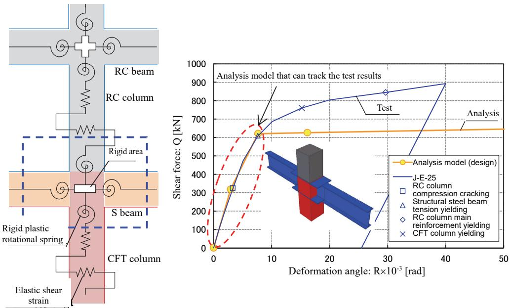
Figure 12. Comparison of analysis model and test results
