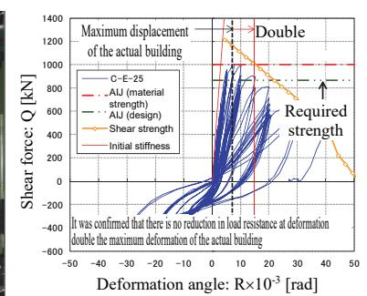
Figure 10. Test specimens and test results
