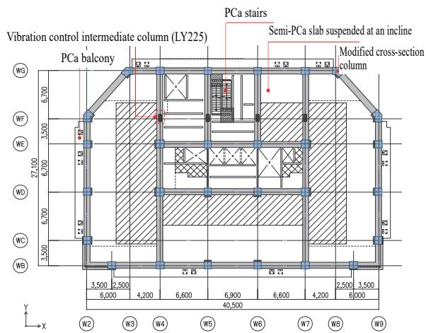
Figure 5. Standard floor framing plan
