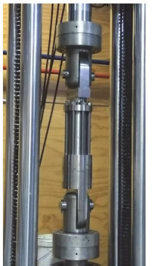
a) Photograph of the damper mounted within the universal test machine during testing.
