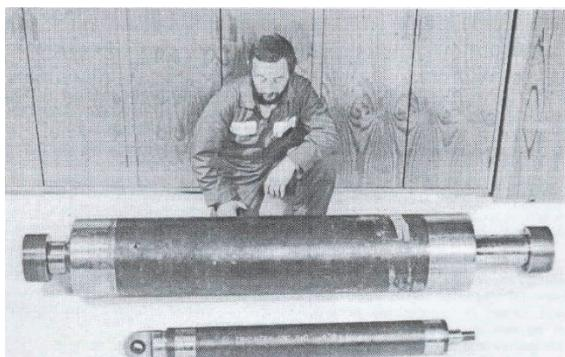
a) Lead extrusion devices developed for base-isolation applications with 100 and 700 kN force capacities. (Cousins and Porritt 1993)
