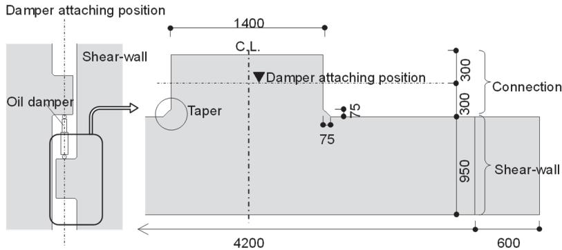
Figure 8. Specimen for cyclic loading test.
