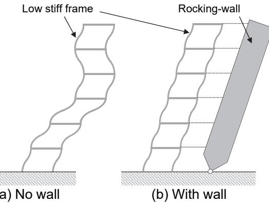
Figure 2. Conceptual diagram of “Shin-bashira effect” of rocking-wall.
