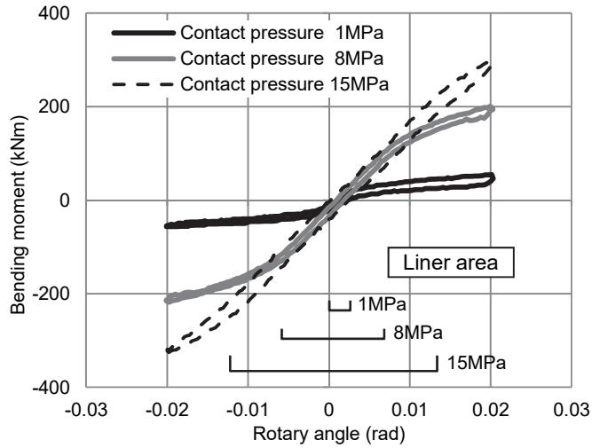
Figure 6. Bending moment–rotary angle relation.
