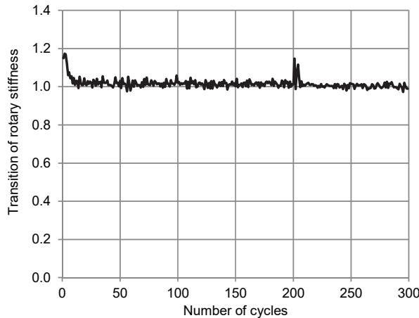
Figure 7. Transition of rotary stiffness (contact pressure: 1MPa).
