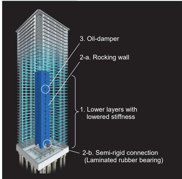
*Figure 1. Perspective drawing of the system.*
