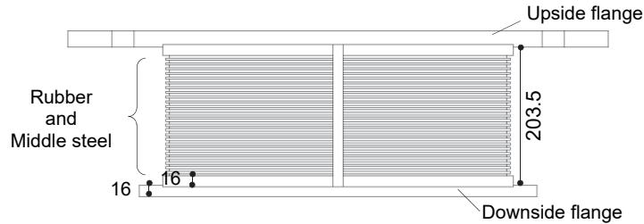
Figure 4. Specimen for rotary deformation test.
