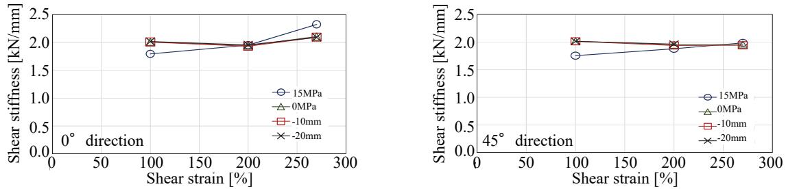
Figure 14. Shear stiffness of seismic isolator.
