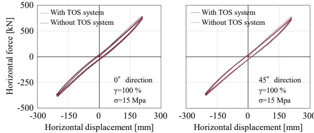
Figure 12. Comparison of cases with and without TOS System.
