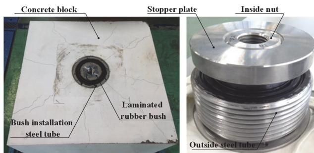
Figure 7. Condition of test specimen (After failure property confirmation test).
