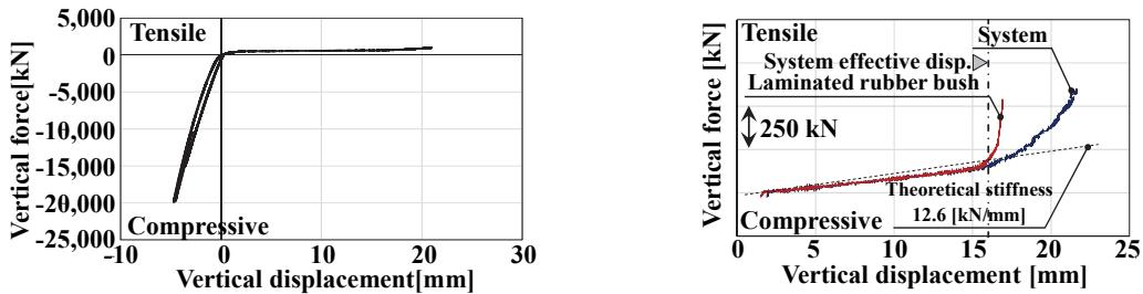
Figure 10. Vertical loading tests and vertical tensile test results.
