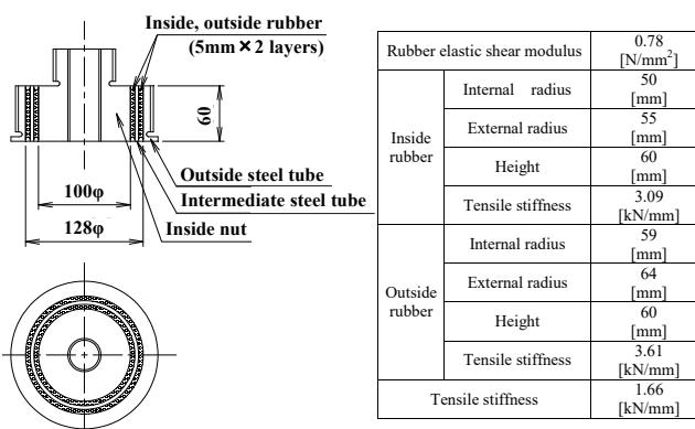
Figure 4. Laminated rubber bush dimensions.
