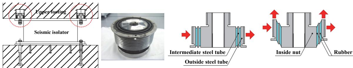
Figure 1. TOS System installation position and outline of the laminated rubber bush.
