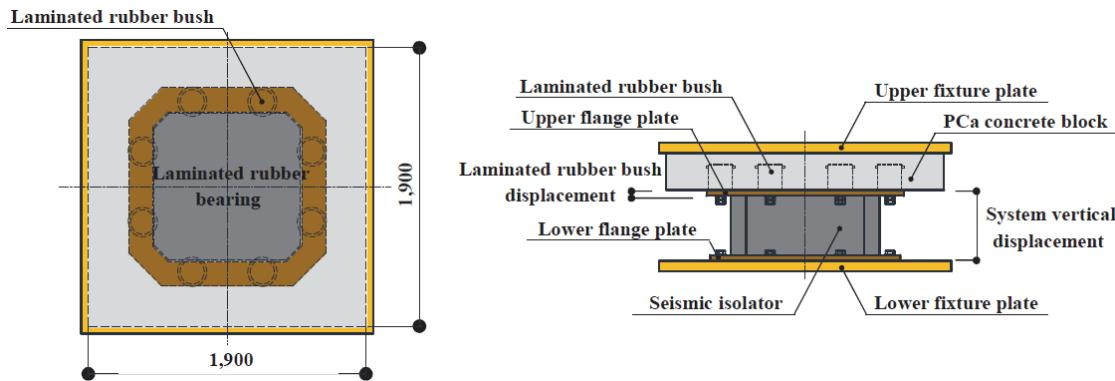
Figure 8. System test specimens.
