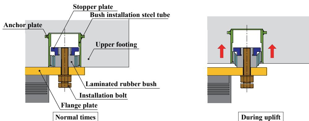
Figure 2. Member configuration of the TOS System.
