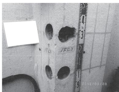
*Photo 6. Investigation of the diameter and material by destructive test.*
