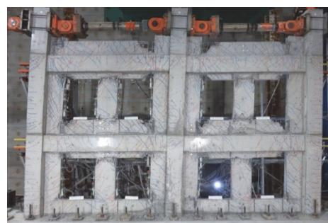
Photo 2. Damage state at  $R=3.0\%$
