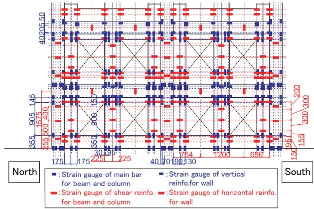
*Figure 8. Strain Gauge Setup*
