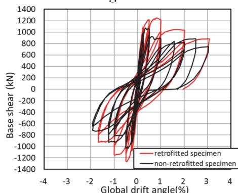
Figure 10. Comparison of Load – Displacement Relationships
