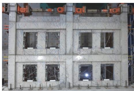
Photo 1. Damage state at  $R=1.0\%$
