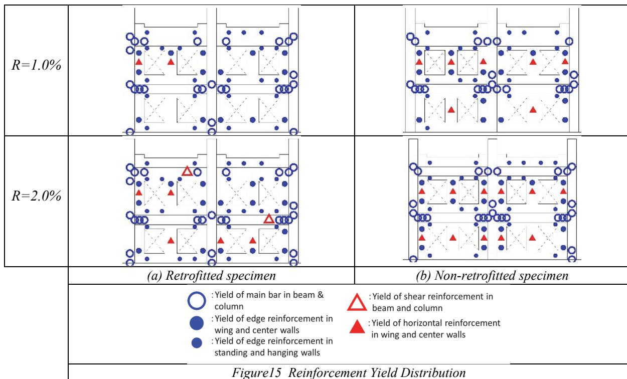
Figure 15 Reinforcement Yield Distribution
