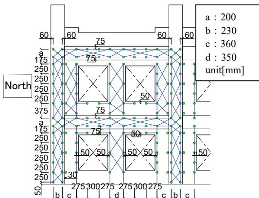
*Figure 7. Displacement Transducer Setup*
