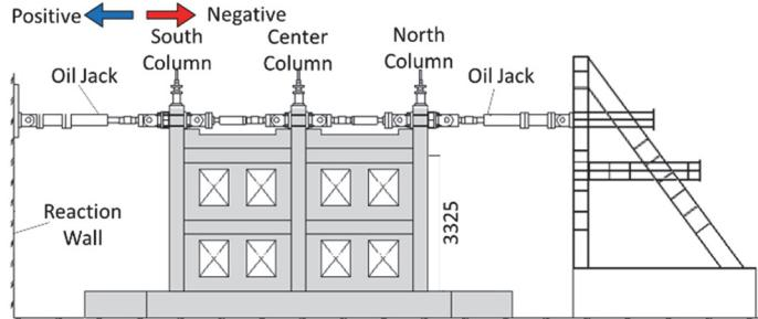
*Figure 5. Loading Setup*
