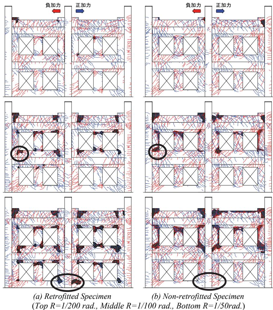
Figure 14. Damage States
