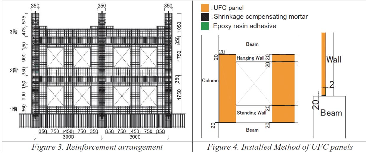
*Figure 3. Reinforcement arrangement*
