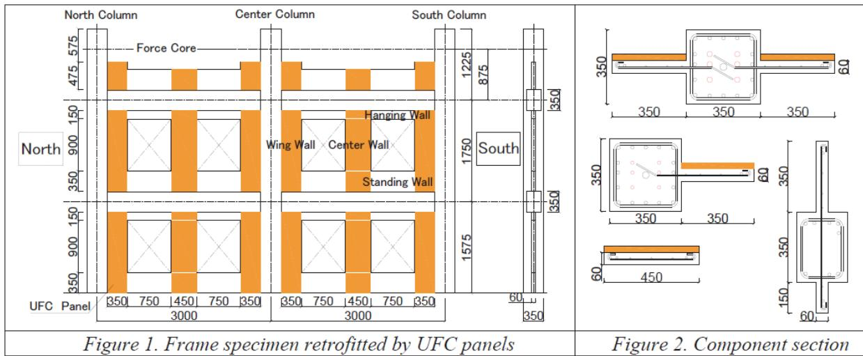
*Figure 1. Frame specimen retrofitted by UFC panels*
