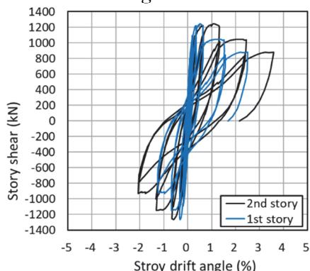
Figure 9. Story Shear and Story Drift Angle Relationships
