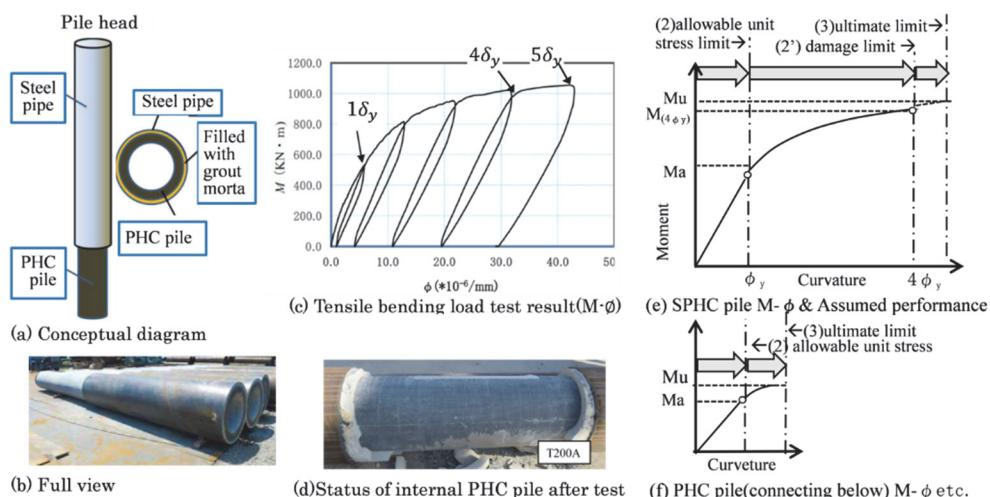
Fig 7. Outline of SPHC pile, its loading test result, seismic performance,
