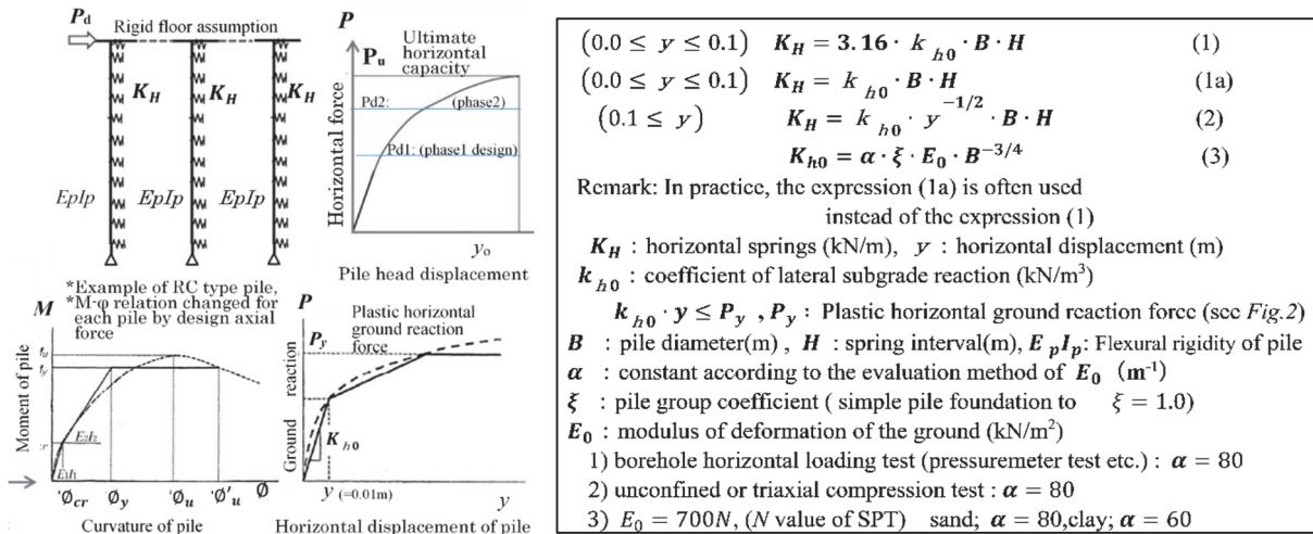
Figure 2. Seismic design model of pile foundation common in practice (leftmost above) the top next; right figure analysis result of  $P$  -  $Y$  relationship of whole pile, leftmost down; model example of flexural stiffness and subgrade reaction of each pile.
