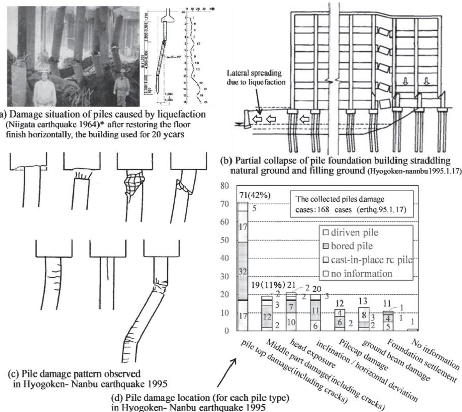
*Figure 1. Earthquake Damage Case of Pile Foundation Building ((a) Niigata1964), (b) Hyogoken-nanbu1995), Related damage investigation Result. ((c) Damage pattern, (d) Damage Position, (d) Survey of damage position of pile.*
