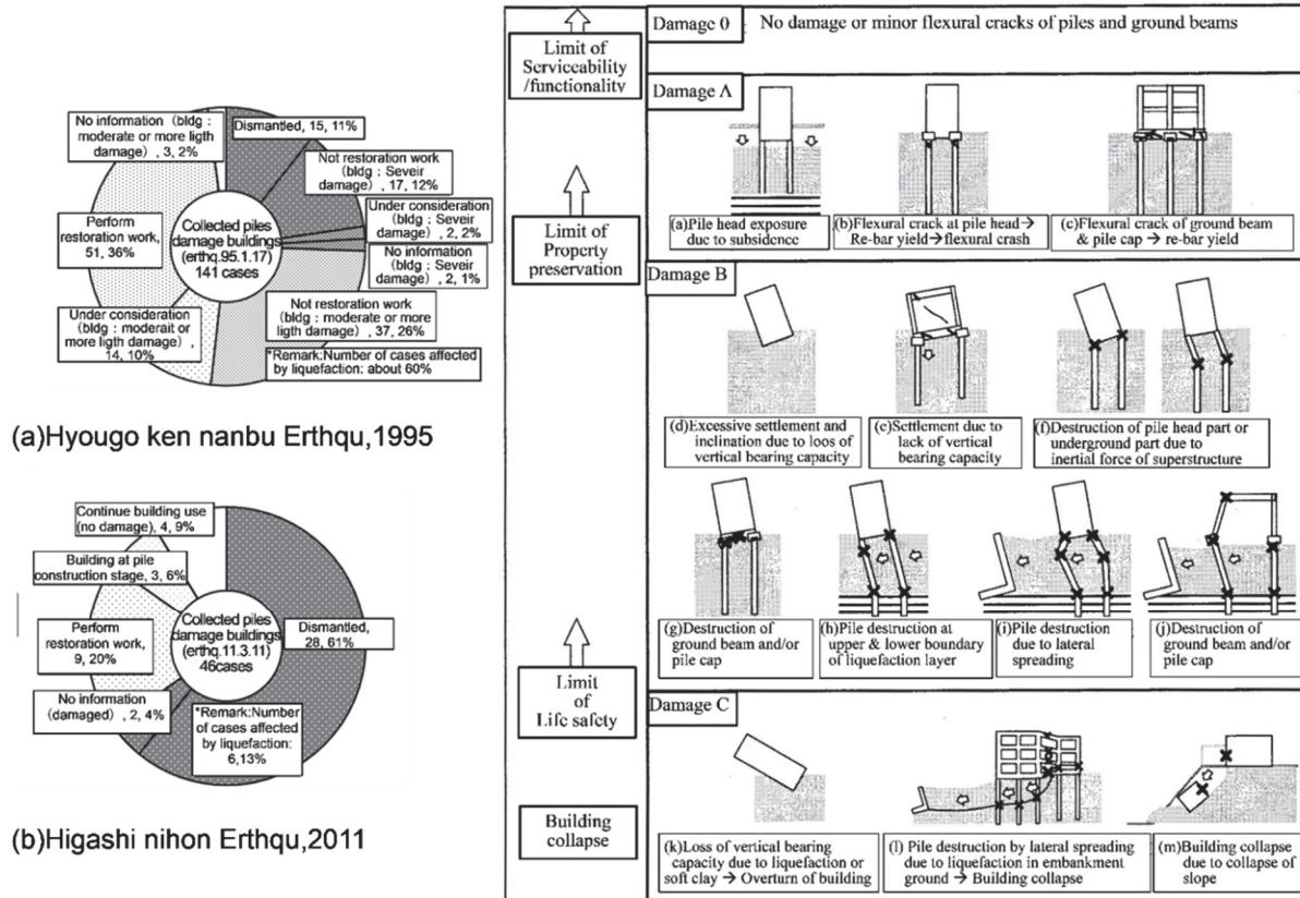
Figure 5. Dismantled / restoration investigation of pile foundation damaged building (EQ1995&2011).
