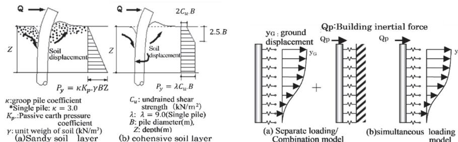
Figure 3. Plastic horizontal subgrade reaction force;  $P_y$ . Fig 4 Pile-ground model for evaluating the influence of ground displacement in addition to the inertial force of the superstructure. (AIJ (2001)).
