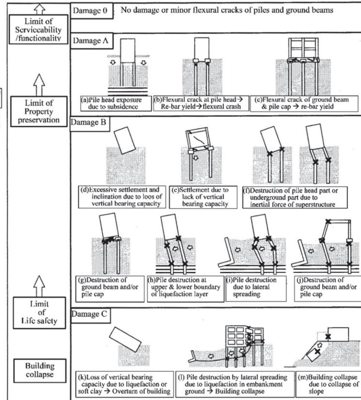
Figure 6. Relationship between damage statuses of pile foundation (EQ 95.1.17) and required performance of building. (Translation of Kobayashi (2001) in Japanese at the author's responsibility.)
