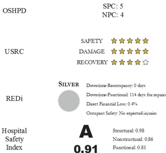
Figure 1. Hospital resilience rating results for four of the rating systems.
