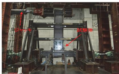
Photo 3. Cyclic loading test on beam.
