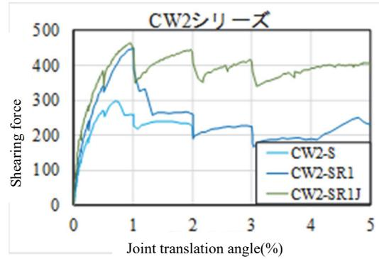
Figure 5. Effectiveness of seismic retrofitting using UFC Panel
