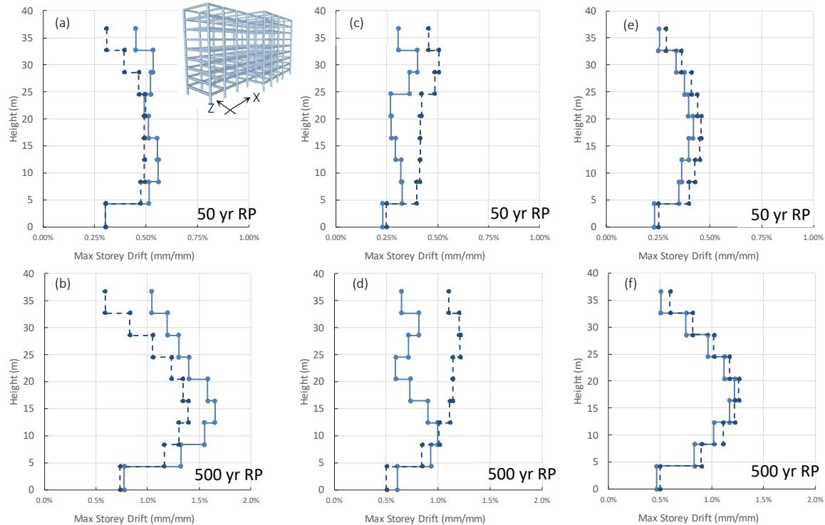
*Figure 6. Average diaphragm centre-of-mass maximum storey drift profiles (a & b) Building 1 ULS design with  $\mu = 4$  typical NZ design (c & d) Building 2 ULS design with  $\mu = 2$  displacement-based ductility evaluated design (e & f) Building 3 SLS 50 year RP design with  $\mu = 1$ .*
