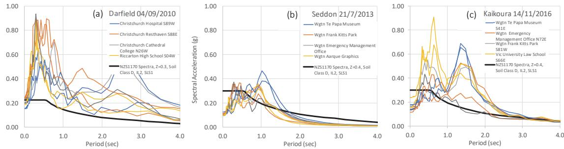
Figure 1. Acceleration spectra for (a) Darfield earthquake recorded in Christchurch (b) Cook Strait earthquake recorded in Wellington (c) Kaikoura earthquake recorded in Wellington.
