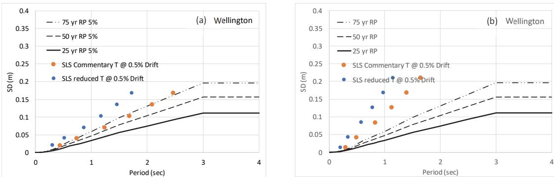
Figure 5 Centre-of-mass response building heights  $n = 2$  to 20. Orange dots represent design to typical ductility (likely  $\mu = 4$  or more), blue dots represent the approximate reduction of design ductility to 1.5-2.5 (a) RC frame approx. elastic period-design displacement points (b) RC shear wall approx. elastic period-design displacement. Allowance for torsion amplification of 20% has been made in determining a reduced centre-of-mass displacement.
