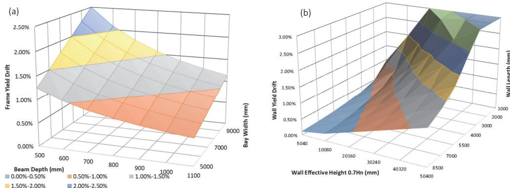
*Figure 3. (a) RC moment-frame nominal yield drift as a function of beam-bay span and depth (b) RC shear-wall nominal yield drift as a function of wall effective height ( $0.7H_n$ ) and wall length. First yield is assumed to typically occur at 65-75% of nominal yield.*
