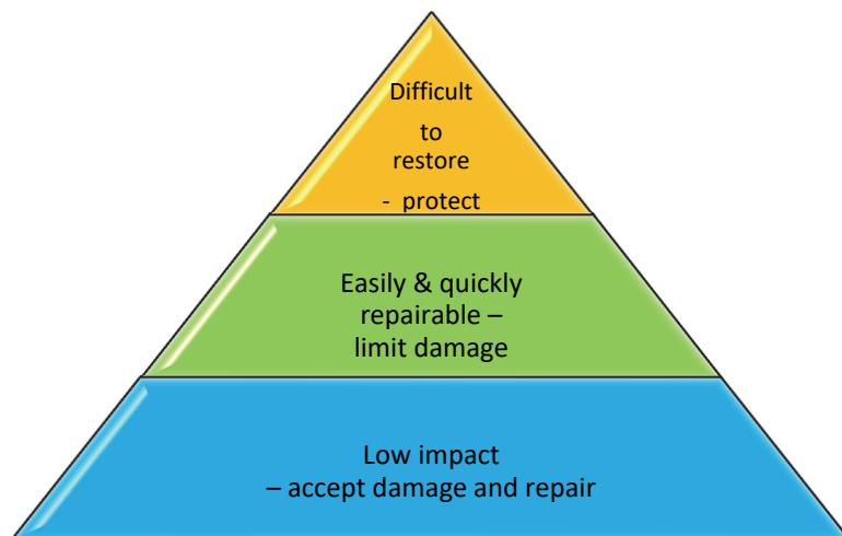
Figure 6. Principles for resilience-based design.
