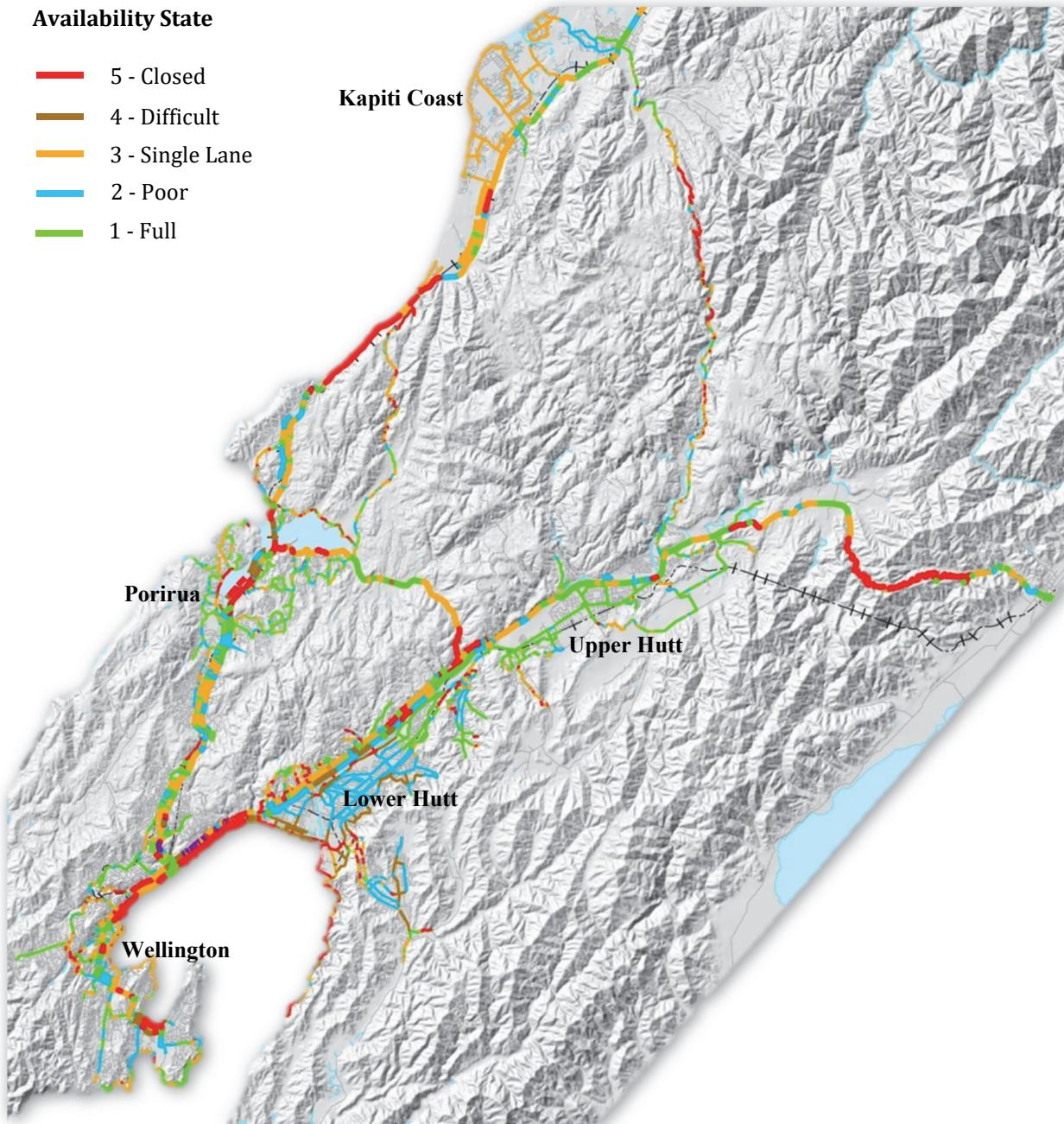
Figure 3. Resilience of Wellington road transport network in a local large earthquake event.
