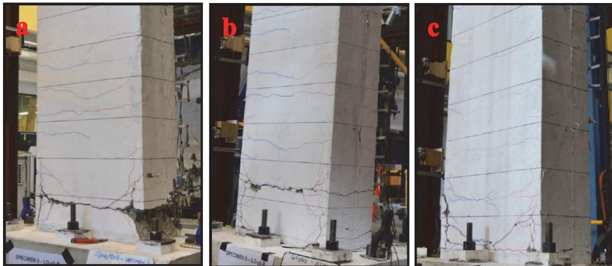
Figure 2. Pre-repair damage state for specimen (a) LD-1-R (b) LD-2-R (c) LD-2-LER-R
