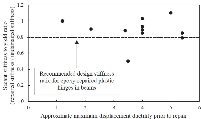
Figure 3. Post-repair secant stiffness to yield ratio vs. maximum displacement Ductility prior to repair.
