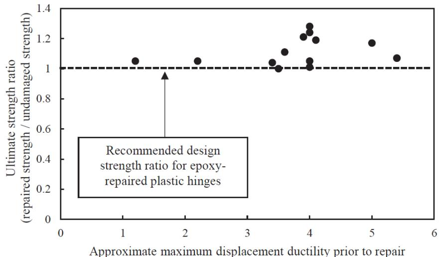
Figure 4. Post-repair ultimate strength ratio vs. maximum displacement Ductility prior to repair.
