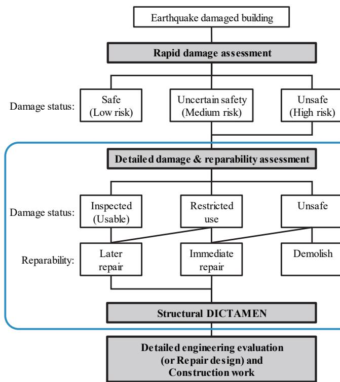
Figure 7. Seismic damage assessment flow.
