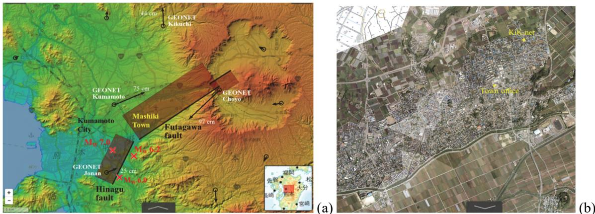
Figure 1. Location of causative faults and GNSS stations in the 2016 Kumamoto earthquake (a) and a mosaiced orthorectified aerial image by GSI and location of seismic stations in Mashiki Town (b)
