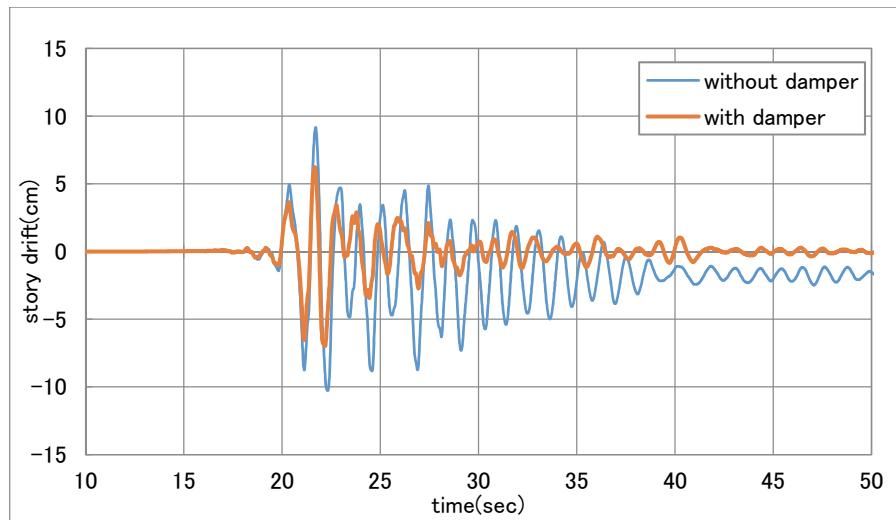
*Figure 10. Story drift of 1st floor.*
