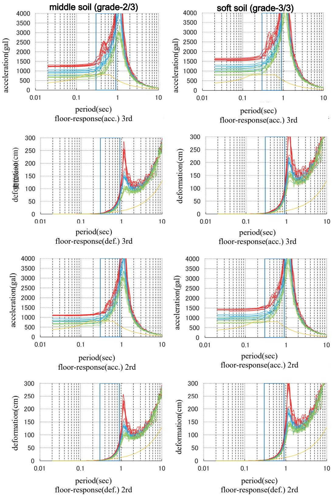
Figure 11. Floor-response for 2nd&3rd floor.
