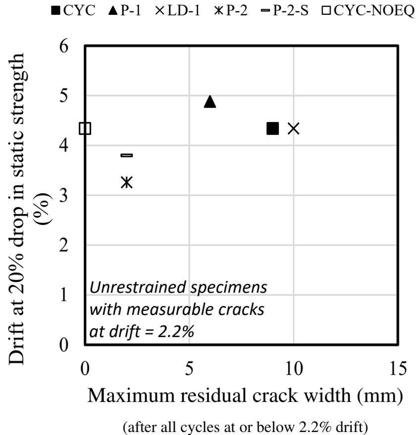
→ No relationship between crack widths and drift capacity.
