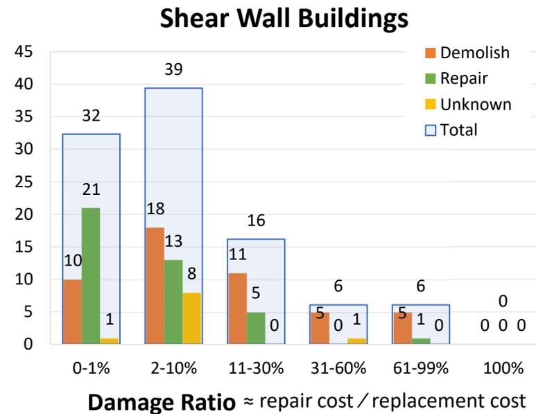
**→ Significant number of RC buildings with relatively low damage were demolished.**
