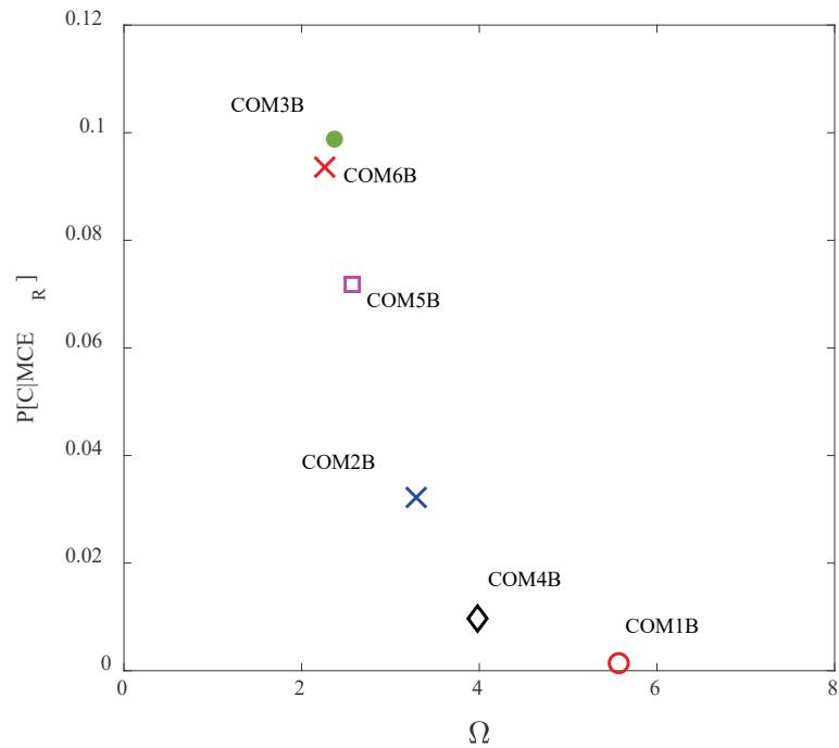
Figure 5-7 MCE<sub>R</sub> collapse probability versus  $\Omega$  for the baseline models.
