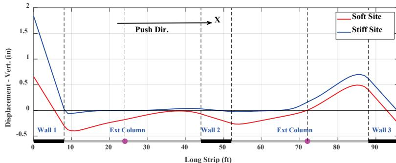
Figure 5-13 Vertical displacements of the foundations for the stiff and soft sites at the respective maximum base shear.
