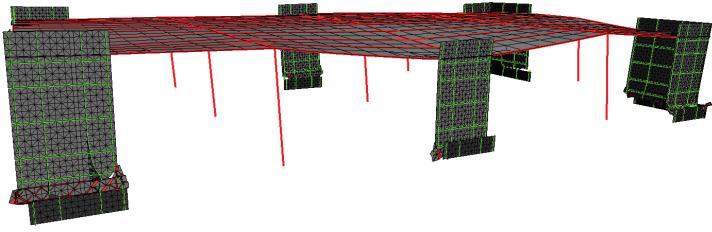
Figure B-37 Deformed meshes from refined model: COM4 (LS-DYNA) – Motion 2 ( $1.8 \times MCE_R$ ).
