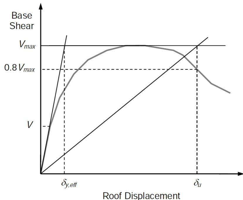
Figure 4-32      Idealized nonlinear static pushover curve (FEMA, 2009b).
