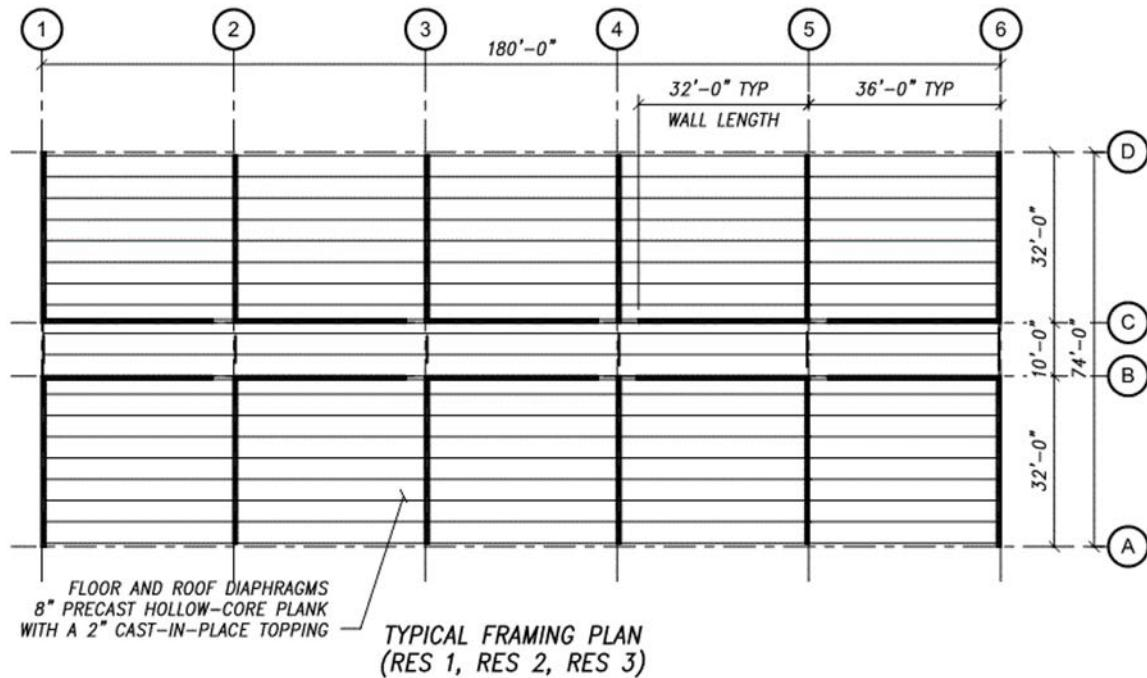
Figure A-39 Four-story residential building framing configuration: RES1, RES2, RES3.
