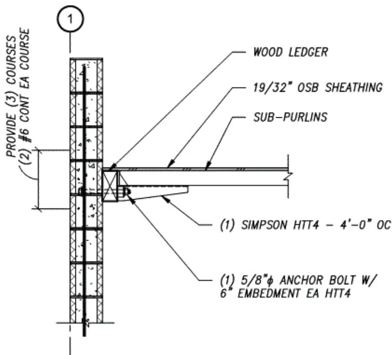
Figure A-62 Single-story retail/industrial/warehouse building framing detail.
