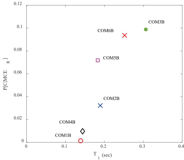
Figure 5-8 MCE<sub>R</sub> collapse probability versus averaged fundamental period for the baseline models.
