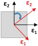
*Axes of orthotropy rotate together with the axes of principal strains*
