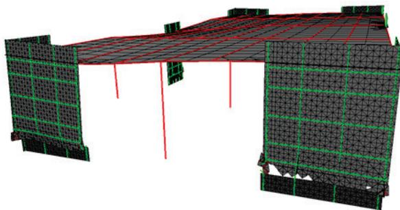
Figure B-38 Deformed meshes from refined model: COM4 (LS-DYNA) – Motion 17 ( $2 \times MCE_R$ ).
