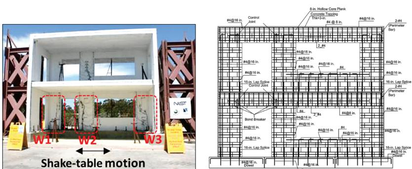
Test configuration and reinforcement details
