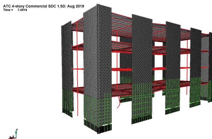
Figure B-60 Deformed meshes from refined model: COM6 (LS-DYNA) – Motion 17 ( $2 \times MCE_R$ ).
