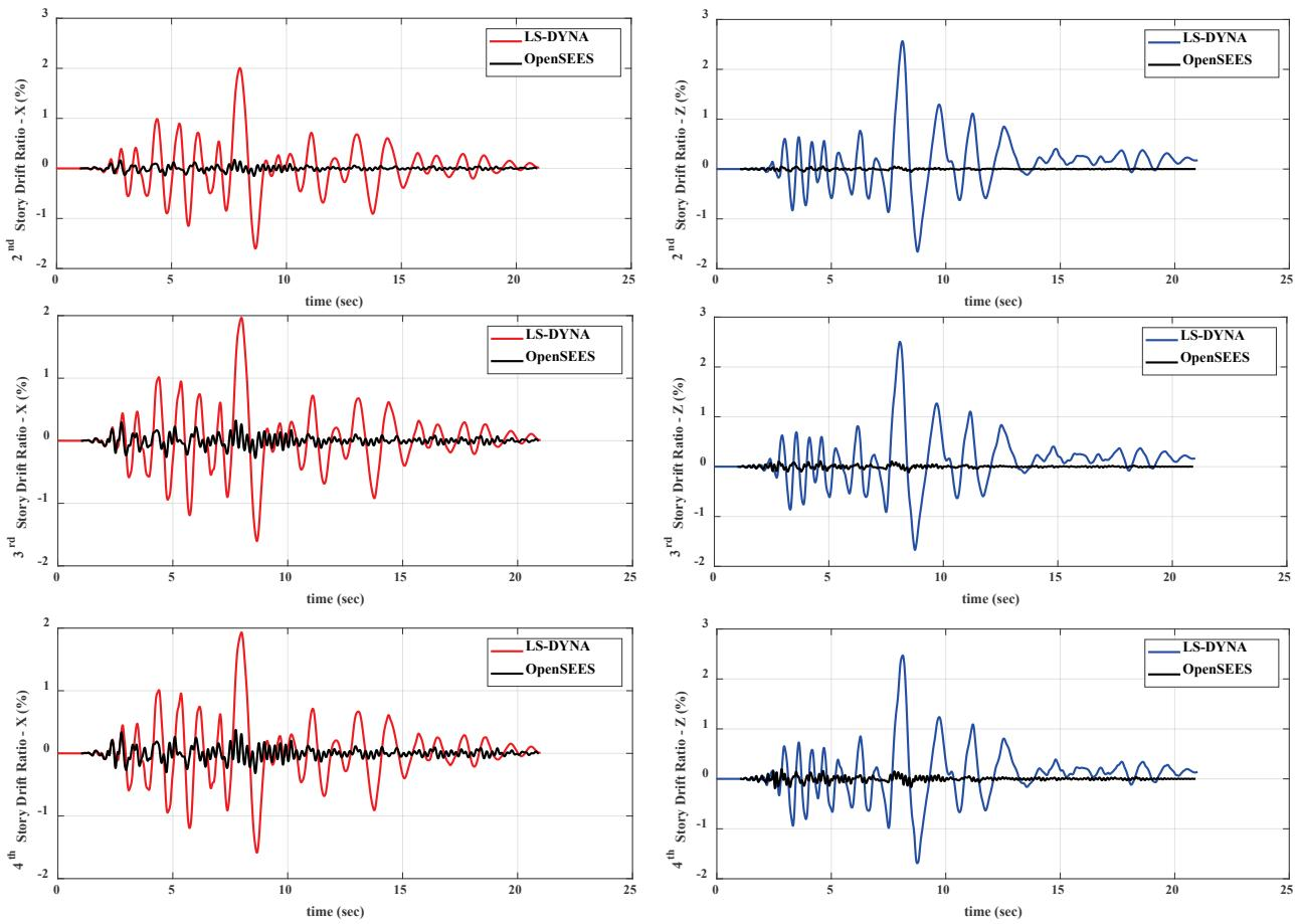
Figure B-32 Comparison of story-drift histories for the upper stories: COM3 – Motion 1 (MCE<sub>R</sub>).
