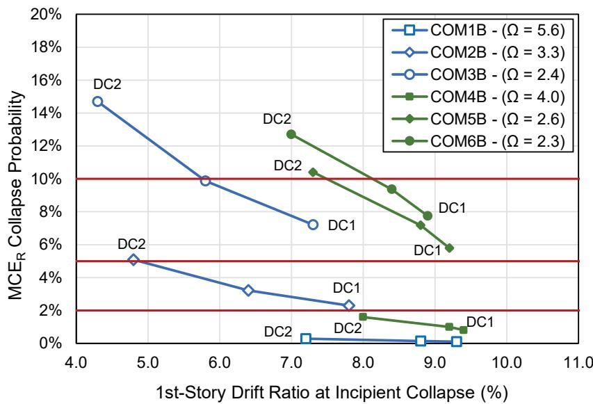
Figure 6-3 MCE<sub>R</sub> collapse probability as a function of first-story drift ratio at incipient collapse of archetype models with varying amounts of post-capping displacement capacity, and benchmark (BM) values of MCE<sub>R</sub> collapse probability and the MCE<sub>R</sub> collapse-safety objective of ASCE/SEI 7-10. Archetype model overstrength ( $\Omega$ ) is shown in the legend.
