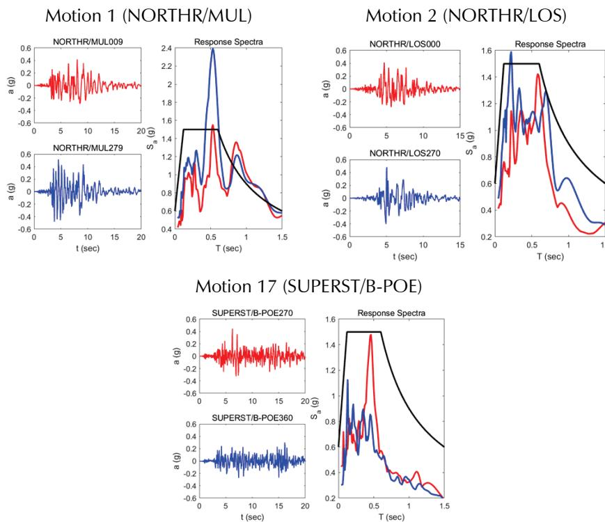
Figure 4-27      Earthquake ground-motion records used for response-history analyses (records shown are unscaled; MCE<sub>R</sub> spectrum is the black solid line).
