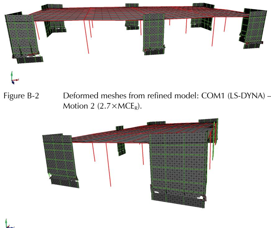
Figure B-2 Deformed meshes from refined model: COM1 (LS-DYNA) – Motion 2 ( $2.7 \times MCE_R$ ).
