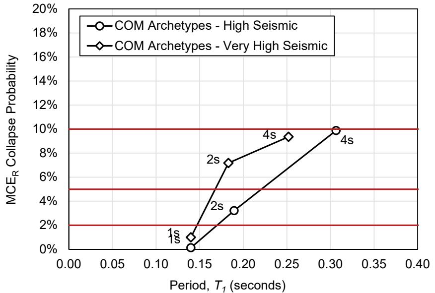
Figure 6-1 MCE<sub>R</sub> collapse probability of baseline archetype models plotted as a function of archetype model period ( $T_1$ ), and benchmark (BM) values of high-seismic MCE<sub>R</sub> collapse probability and the MCE<sub>R</sub> collapse-safety objective of ASCE/SEI 7-10.
