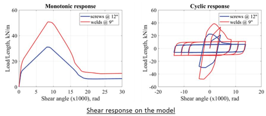
Figure 4-22 Modeling of roof diaphragm.
