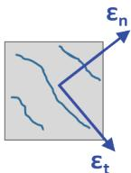
*Axes of orthotropy remain fixed, parallel and normal to the direction of the first crack.*
