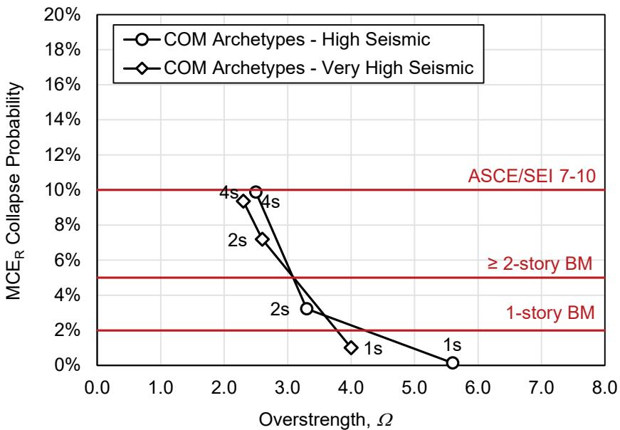
Figure 6-2 MCE<sub>R</sub> collapse probabilities of baseline archetype models plotted as a function of average archetype model overstrength ( $\Omega$ ), and benchmark (BM) values of MCE<sub>R</sub> collapse probability and the MCE<sub>R</sub> collapse-safety objective of ASCE/SEI 7-10.
