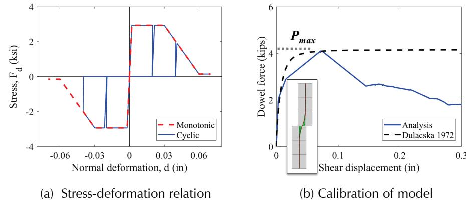
Figure 4-12 Monotonic and cyclic behaviors of dowel-action model.
