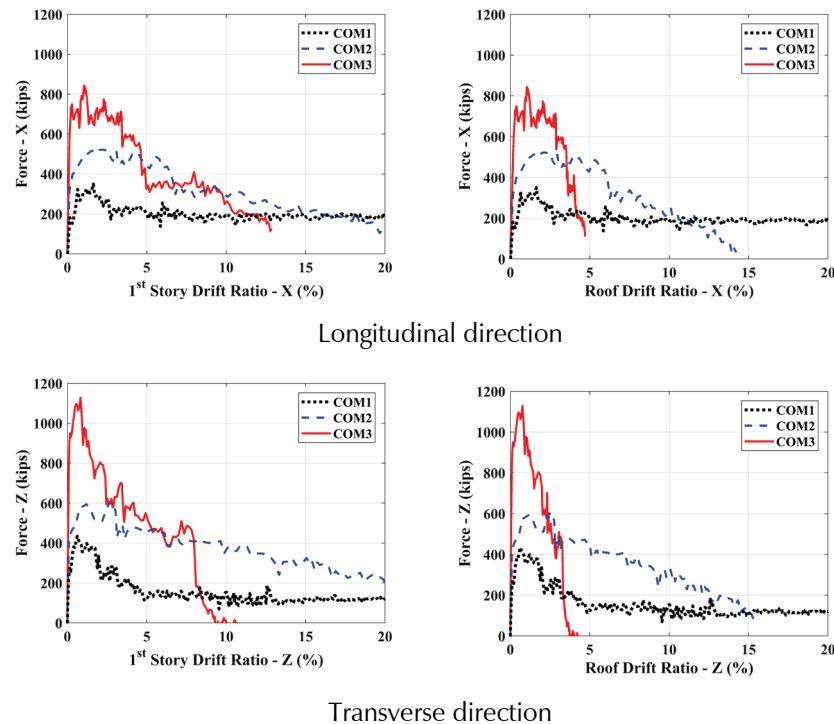
Figure 4-23      Base shear-vs.-story-drift ratio curves for high-seismic archetypes.
