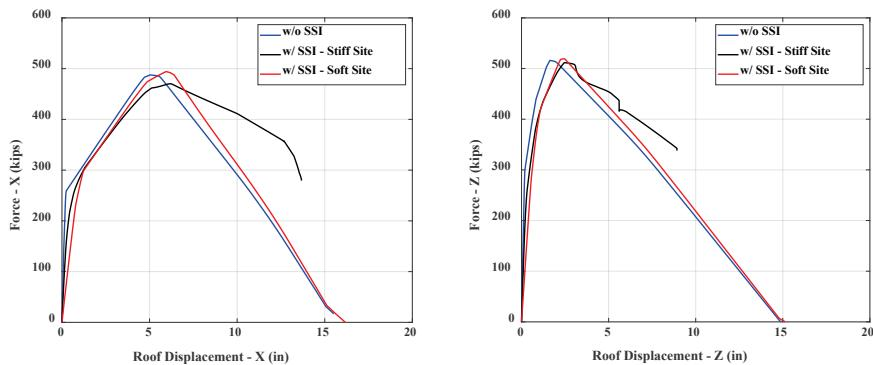
Figure 5-12 Pushover curves for COM2B with and without soil springs and dampers.
