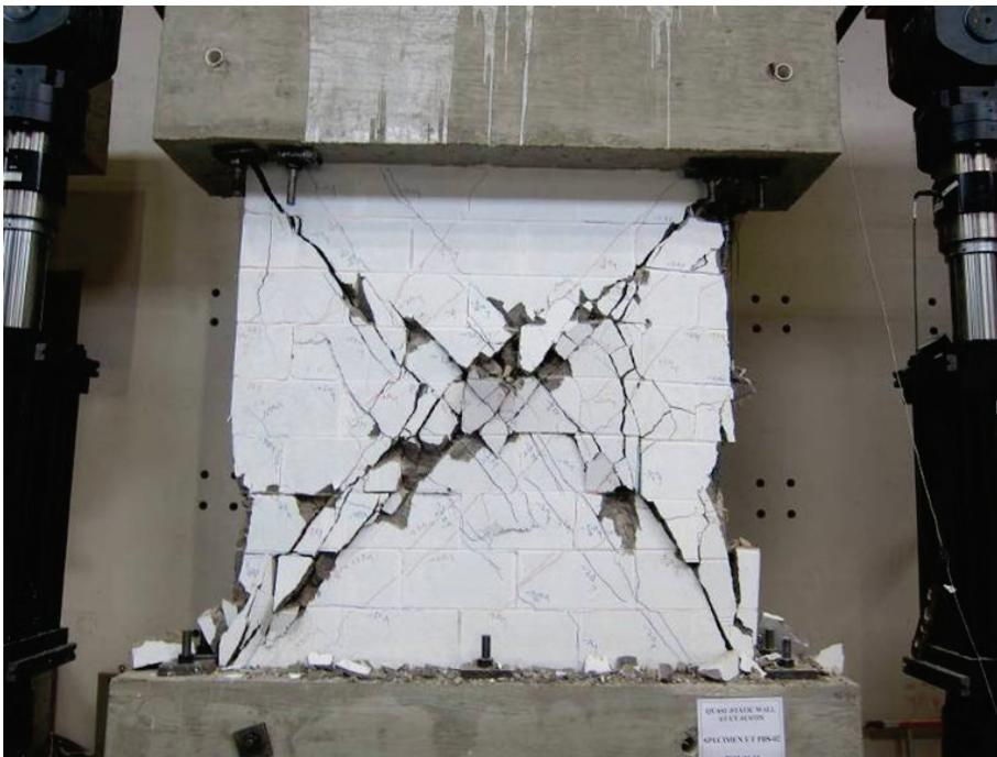
Figure 4-2      Failure of a shear-dominated wall (Wall UT-PBS-02
