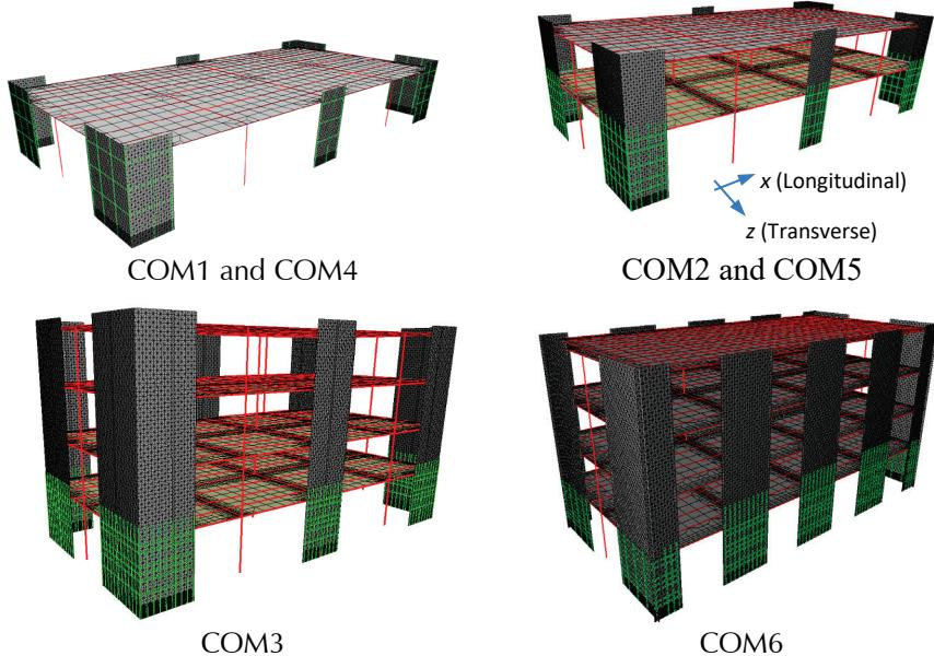
Figure 4-20 Finite-element models for commercial building archetypes.
