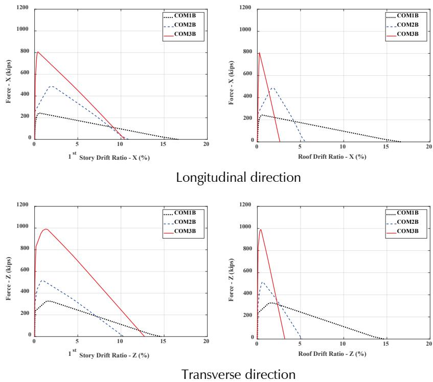
Figure 5-1      Pushover curves for high-seismic baseline models (COM1B, COM2B, and COM3B).
