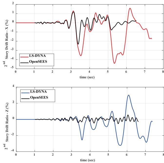
Figure B-20 Comparison of story-drift histories for the second story: COM2 – Motion 2 ( $2 \times MCE_R$ ).
