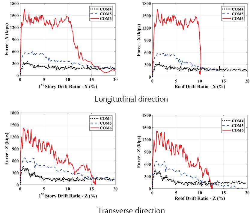
Figure 4-24      Base shear-vs.-story-drift ratio curves for very high-seismic archetypes.
