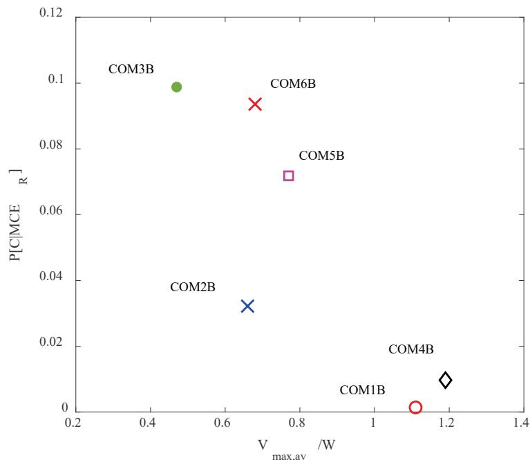
Figure 5-6 MCE<sub>R</sub> collapse probability versus  $V_{max,av}/W$  for the baseline models.
