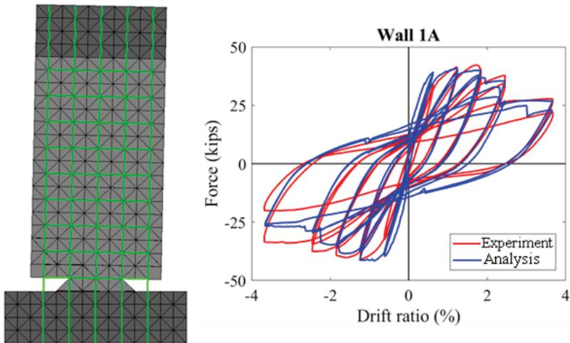
Figure 4-15 Flexure-dominated wall tested by Sherman (2011).
