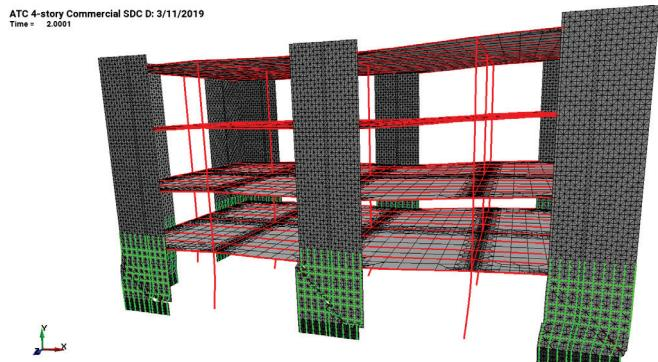
Figure 4-25 Deformed finite-element mesh for COM3 from pushover analysis.
