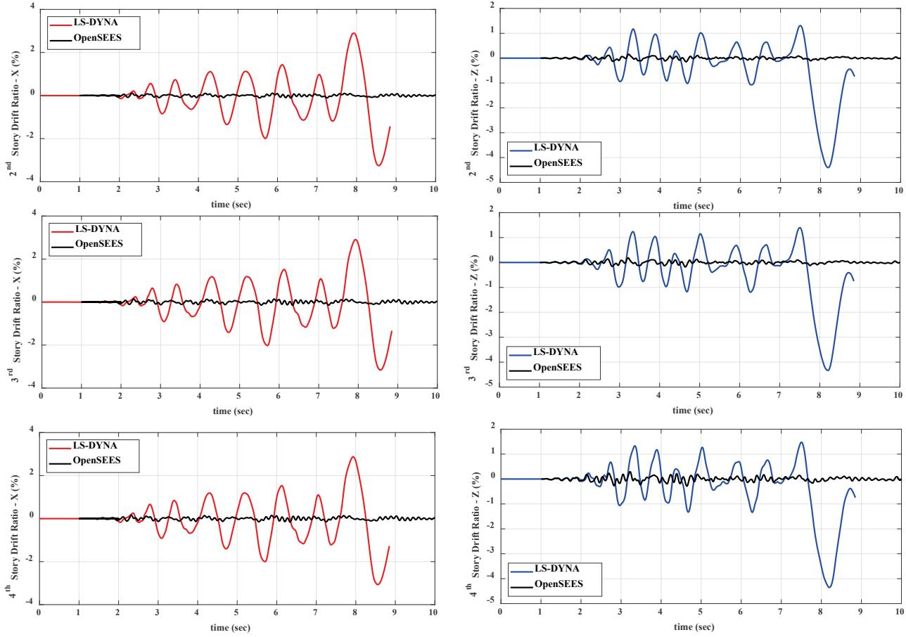
Figure B-67 Comparison of story-drift histories for the upper stories: COM6 – Motion 1 (MCE<sub>R</sub>).
