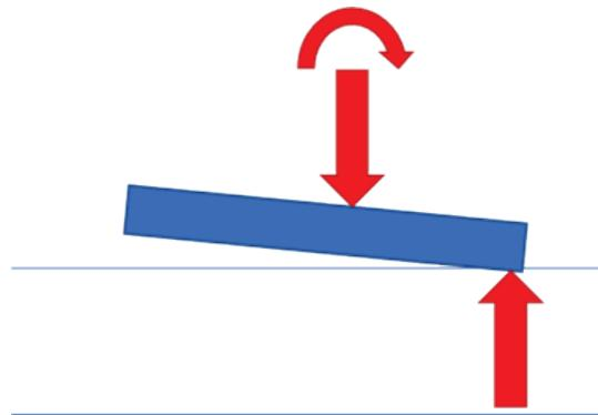
Figure C-3 Equilibrium estimation of rotational capacity of foundation.
