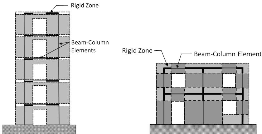
Figure 4-3 Frame models for masonry wall systems.
