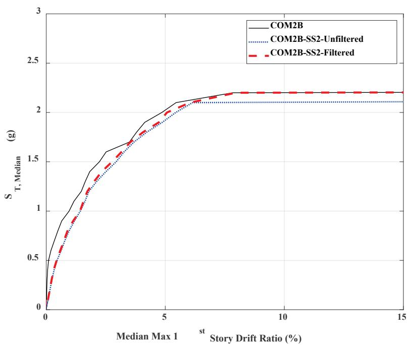
Figure 5-17 Median spectral intensity versus median maximum first-story drift.
