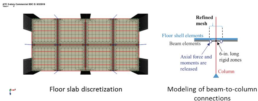
Figure 4-21 Modeling of floor diaphragms.
