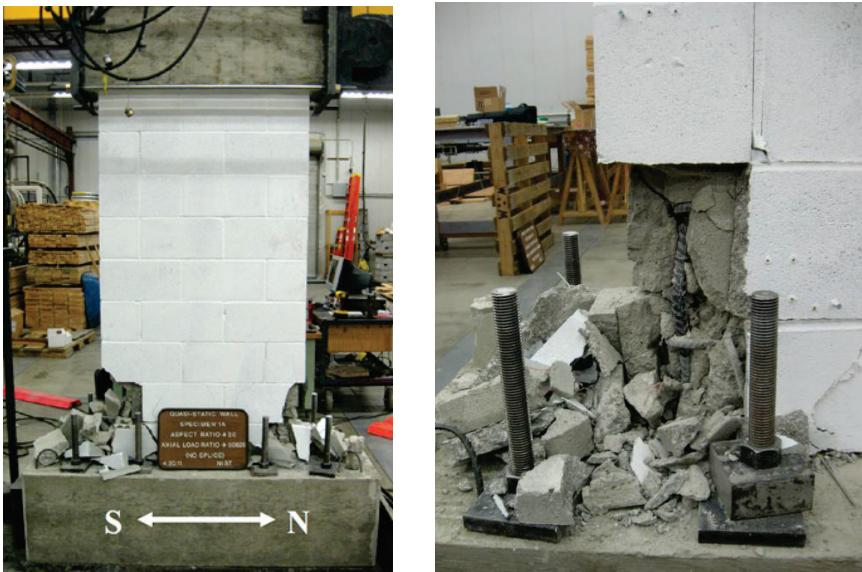
Figure 4-1      Crushing and bar buckling in a flexure-dominated wall
