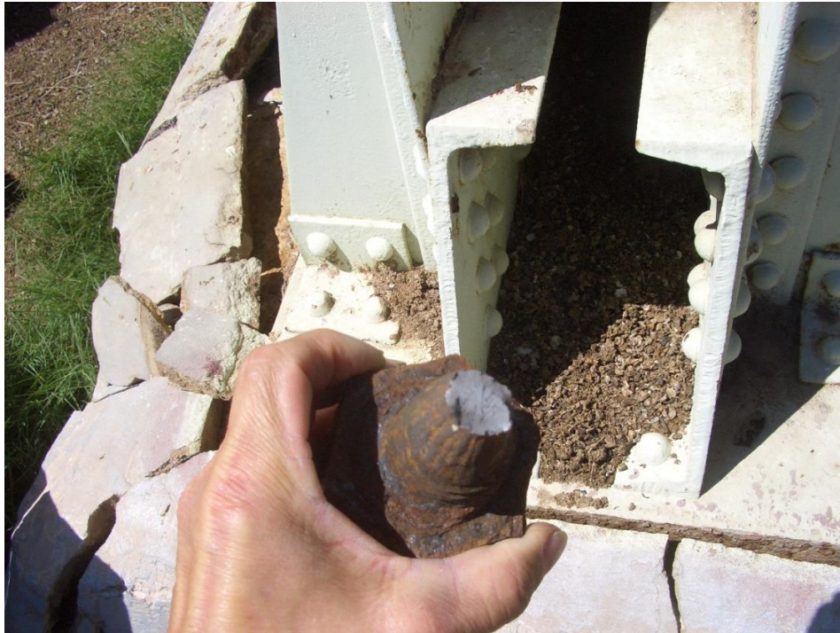
Figure 2-27 – Drawn and snapped connector at footing of water tower, also note footing damage
