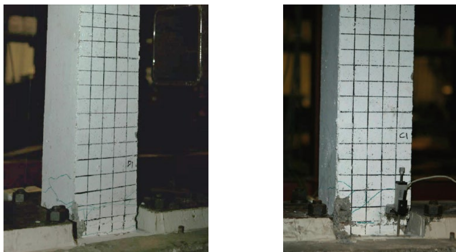
Figure 3-7 Column D1 (left) and Column C1 (right) after Dynamic Test 1 at base.
