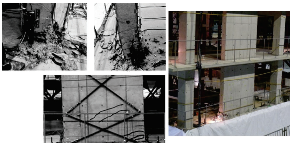
Figure 4-9 Observed damage in first story of shear walls (adapted from Nagae et al., 2015). Top left photos: base of wall at Gridline C closer to Gridline 2 (left) and Gridline 1 (right); Bottom left photo wall base at Gridline A; Photo on the right shows wall at Gridline C.
