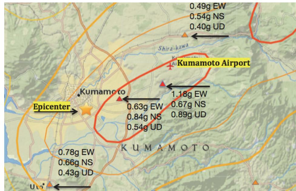
Summary of the ground motions recorded nearest to the Kumamoto Airport. The PGAs for the three components of each record are shown. The map also shows the intensities of the earthquake estimated by the USGS. The area within the red contour is MMI IX; the area within the wider orange contour is MMI VIII. The airport is in MMI IX.
