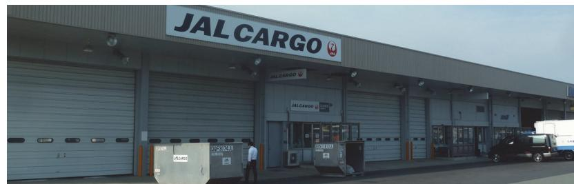
The airport has several steel framed warehouses, hangars, and other service buildings. None appeared to have significant structural damage, including older steel structures that were designed and built to outdated codes. Over time, and in many earthquakes these types of structures, have proven to be much lower risk than comparable concrete frame, precast or tilt-up, and shear wall structures.
