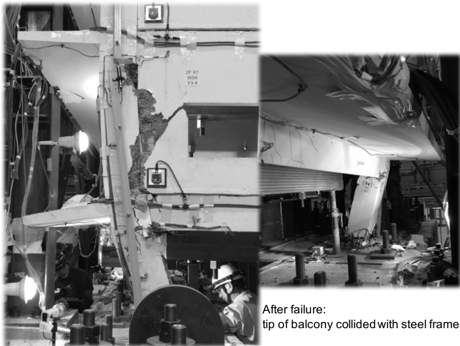
#3-5(JMA Kobe 140%-1) 1/2 wall in X-2 frame on the 2nd floor
