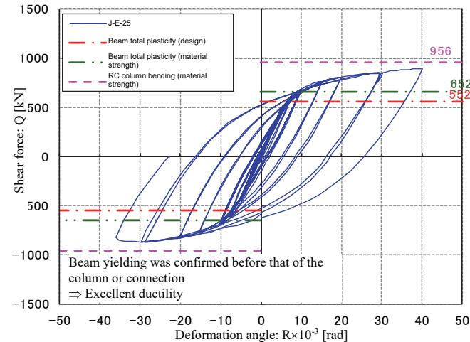
Figure 11. Test specimens and test results (connection tests)
