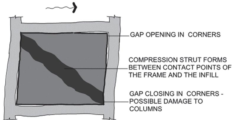
Figure 4. Infill wall subsystem. Note criticality of size of gap.
