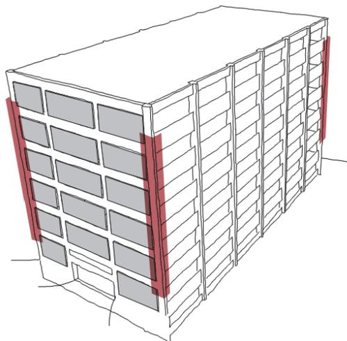
*Figure 3. General form of the smaller building. Critical columns are highlighted red and infill walls in grey*
