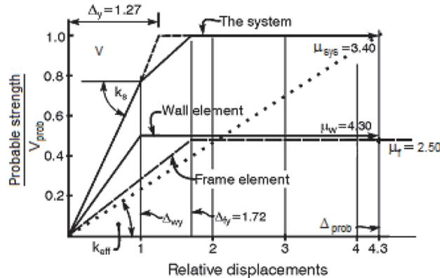
Figure 1. Sample SLaMA backbone curve, (MBIE Seismic Assessment Guidelines)
