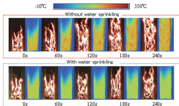
*Figure 4. The difference of flame spreading in a wall surface by watering.*
