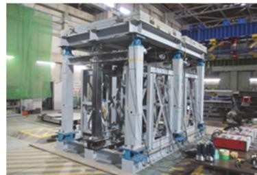
Photo 4. Shaking table test on two-bay frame.
