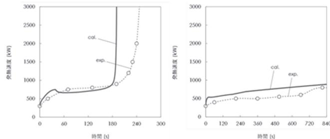
*Figure 3. fire development by the difference of a room interior lining
