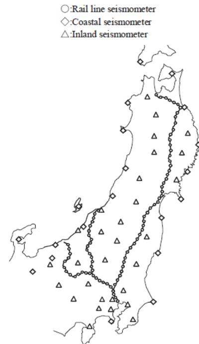
Figure 3 Installation of seismometers <sup>2)</sup>
