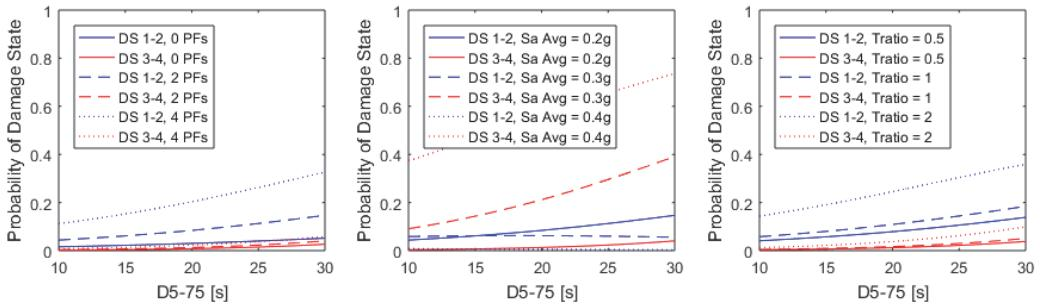
Figure 3. Regression curves for base case: Unretrofit building; End building; Transition Zone; Number of performance factors = 2; Period Ratio = 1; Sa Avg. = 0.2g; Pre-1985; 4-9 stories.
