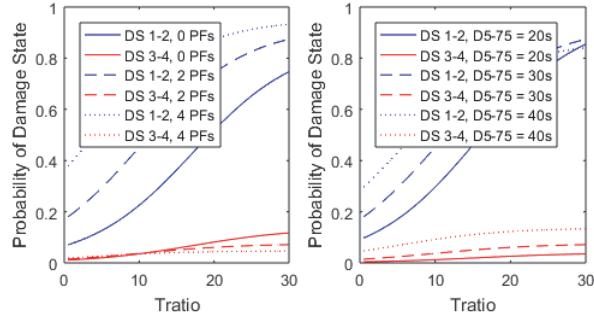
Figure 2. Regression curves for base case: Unretrofit building; Not an end building; Lakebed Zone; D5-75 = 30 seconds; Number of performance factors = 2; Sa Avg. = 0.4g; Pre-1985; 4-9 stories.
