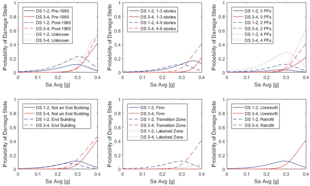
Figure 1. Regression curves for base case: Unretrofit building; Not an end building; Transition Zone; D5-75 = 15 seconds; Number of performance factors = 2; Period ratio = 1; Pre-1985; 4-9 stories.
