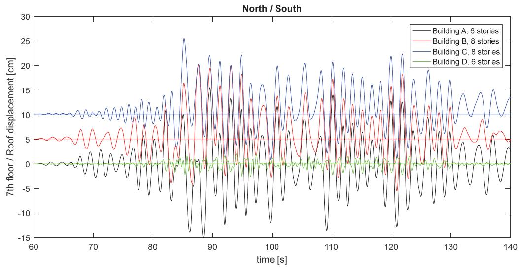
Figure 6. North / South direction top pounding level displacement response histories.
