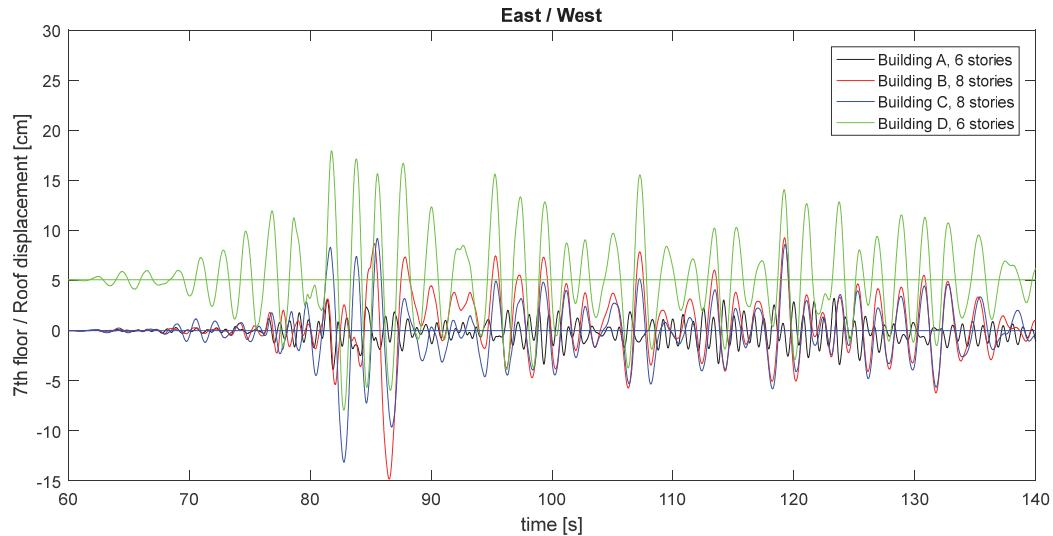
Figure 7. East / West direction top pounding level displacement response histories.
