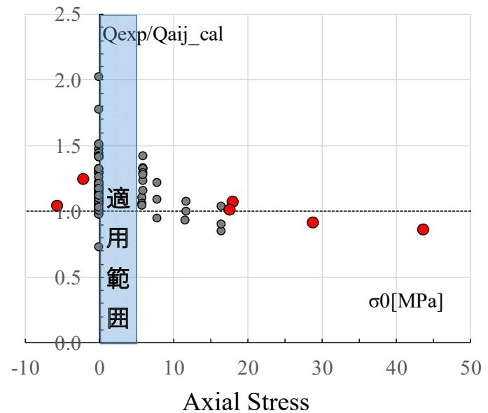
In order to evaluate the shear capacity of precast concrete pile, static loading test was conducted using 9 precast concrete pile specimens.
