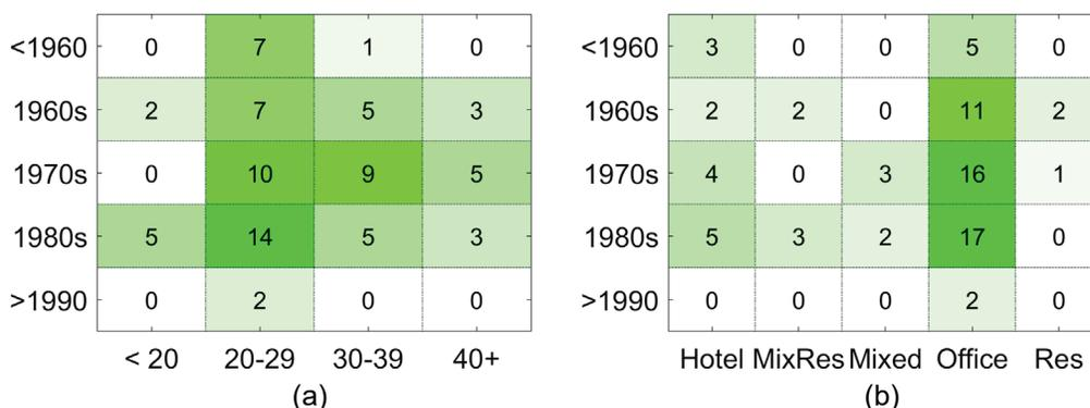
Figure 1-8 Joint distribution of pre-1994 steel moment-resisting frame tall buildings for (a) building date versus number of stories, and (b) date versus occupancy type (values and color intensity denote the number of buildings in each category).
