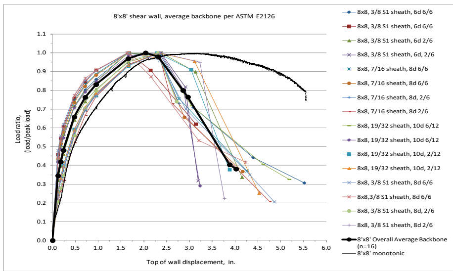
Figure 4-5 Plot of available test data for wood structural panel shear walls with an aspect ratio of one and tie-downs (Line, 2016). Shown in the heavy black line is the recommended normalized curve.
