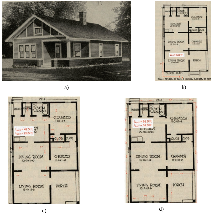
Figure 6-4 Example of one-story 1910 configuration measurements within FEMA P-1100 cripple wall dwelling superstructure study: (a) exterior view of house; (b) plan configuration; (c) plan measured for interior walls; (d) plan measured for exterior walls.
