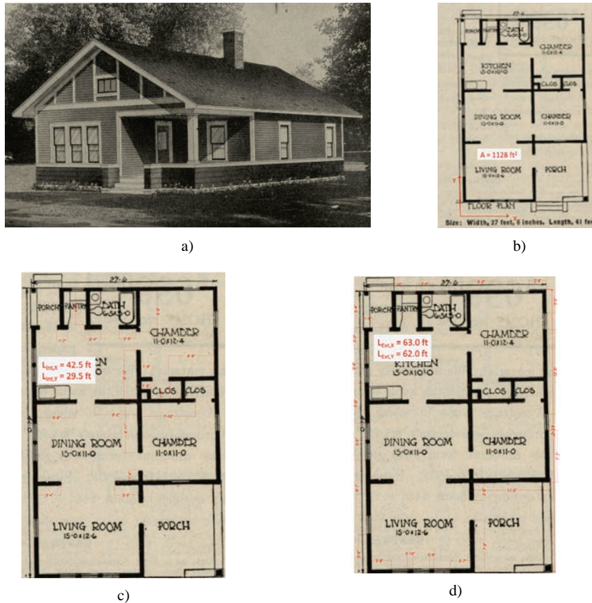
Figure 11-2 Example of one-story 1910 configuration measurements within ATC-110 cripple wall dwelling superstructure study: a) Exterior view of house; b) Plan configuration; c) Plan measured for interior walls; d) Plan measured for exterior walls.
