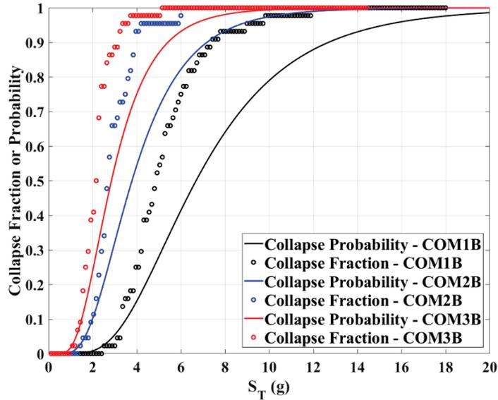
Figure 5-4 Collapse rates from IDA data and collapse fragility curves derived for high-seismic baseline models.  $S_T$  for the collapse fraction data has been scaled by 1.2, whereas that for the collapse probability curve has been scaled by  $1.2 \times SSF$ .
