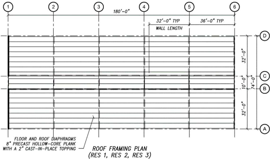
Figure A-40 Four-story residential building roof configuration: RES1, RES2, RES3.
