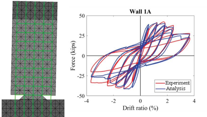
Figure 4-15 Flexure-dominated wall tested by Sherman (2011).
