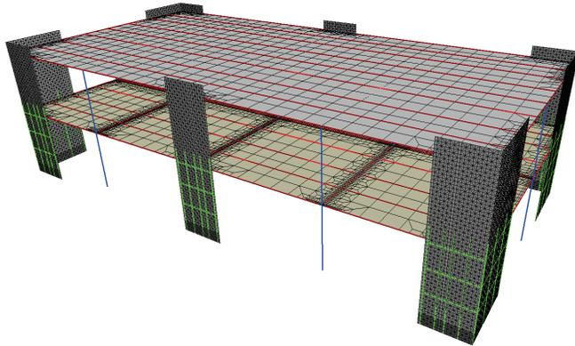
Figure 4-4 Refined finite-element model for a two-story reinforced masonry commercial building archetype.
