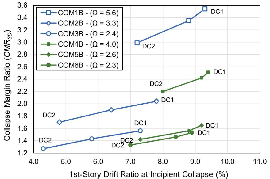
Figure 6-4 Collapse margin ratio ( $CMR_{3D}$ ) as a function of first-story drift ratio at incipient collapse of archetype models with varying amounts of post-capping displacement capacity, and benchmark (BM) values of  $MCE_R$  collapse probability and the  $MCE_R$  collapse-safety objective of ASCE/SEI 7-10. Archetype model overstrength ( $\Omega$ ) is shown in the legend.
