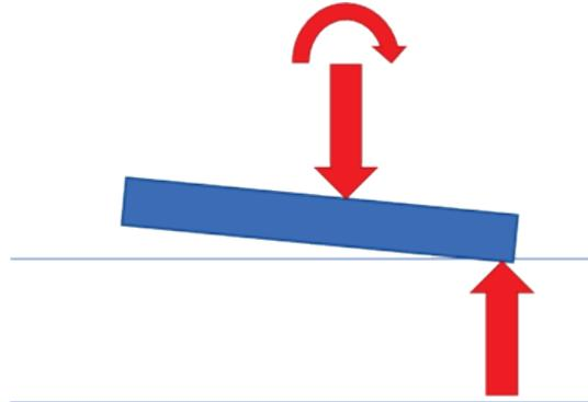
Figure C-3 Equilibrium estimation of rotational capacity of foundation.
