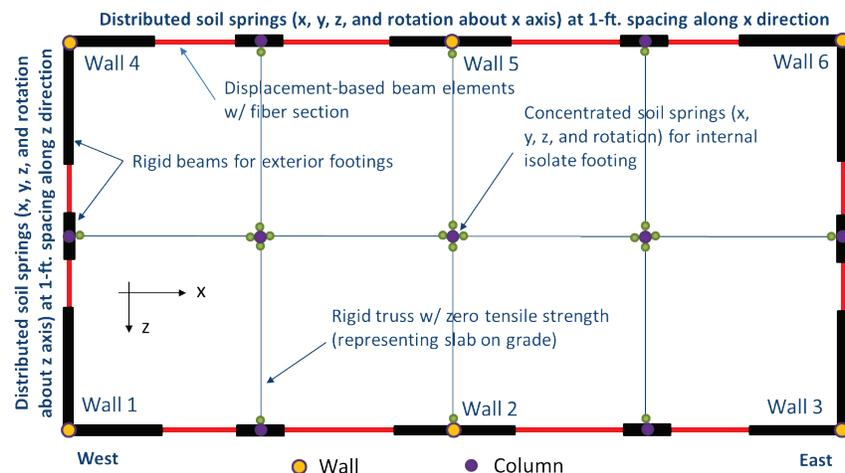
Figure 4-36 Foundation model for the stiff site for SSI analyses.
