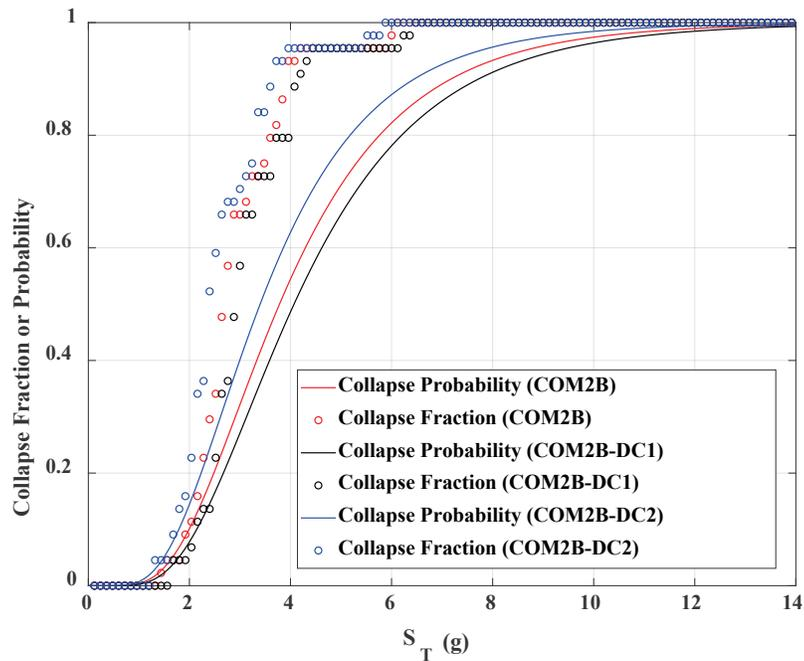
Figure 5-9 Collapse rates from IDA data and collapse fragility curves derived for COM2B, COM2B-DC1, and COM2B-DC2.  $S_T$  for the collapse fraction data has been scaled by 1.2, whereas that for the collapse probability curve has been scaled by  $1.2 \times SSF$ .
