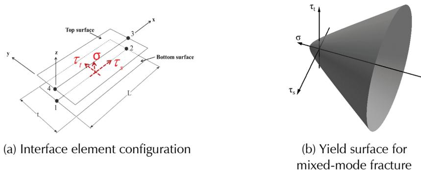
Figure 4-8 Cohesive-crack interface element.
