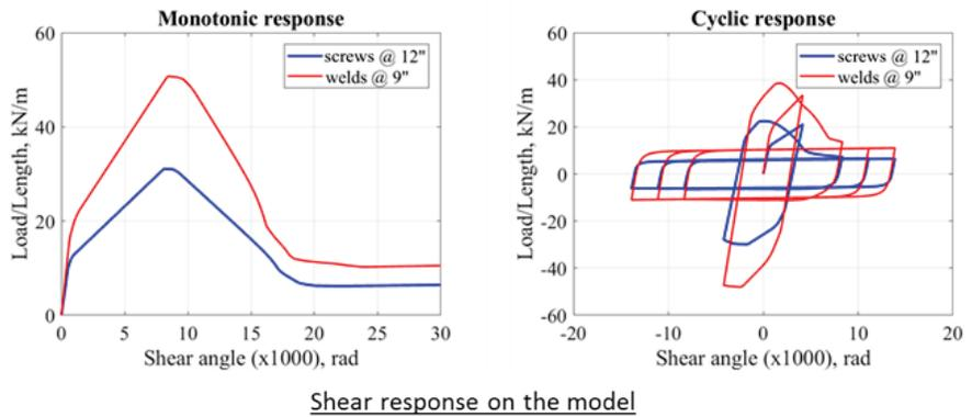
Figure 4-22 Modeling of roof diaphragm.
