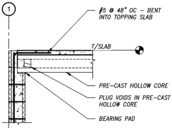
Figure A-50 Residential building framing detail.
