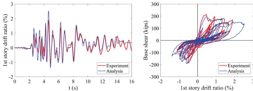
Comparison of experimental and numerical response in the final motion
