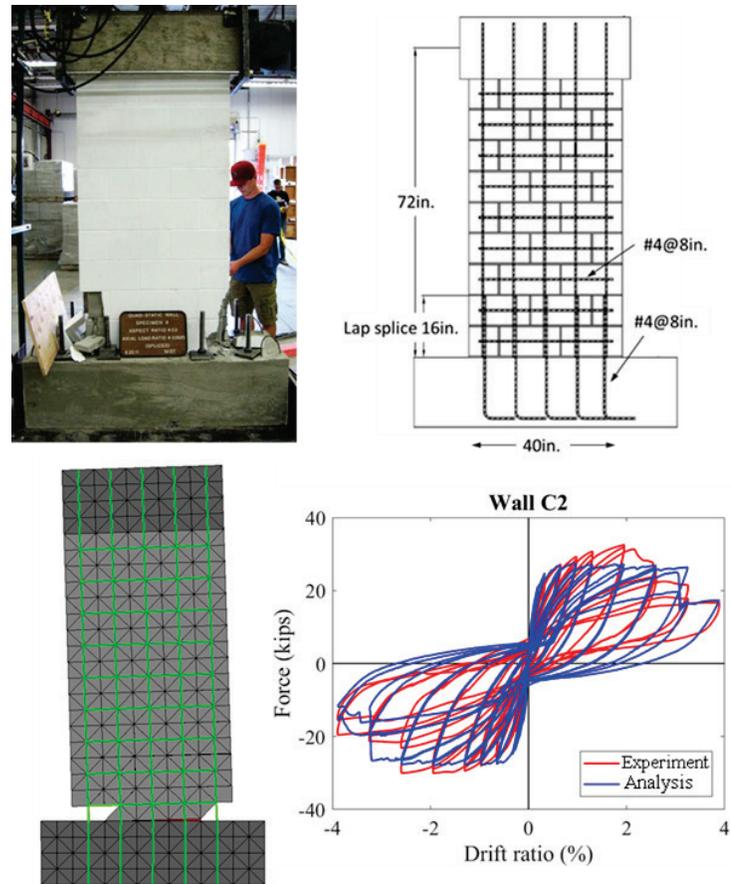
Figure 4-14 Flexure-dominated wall tested by Kapoi (2012).
