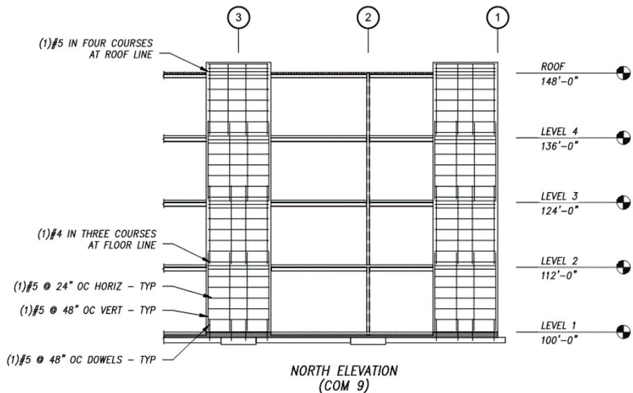
Figure A-25 Four-story commercial building North elevation: COM9.
