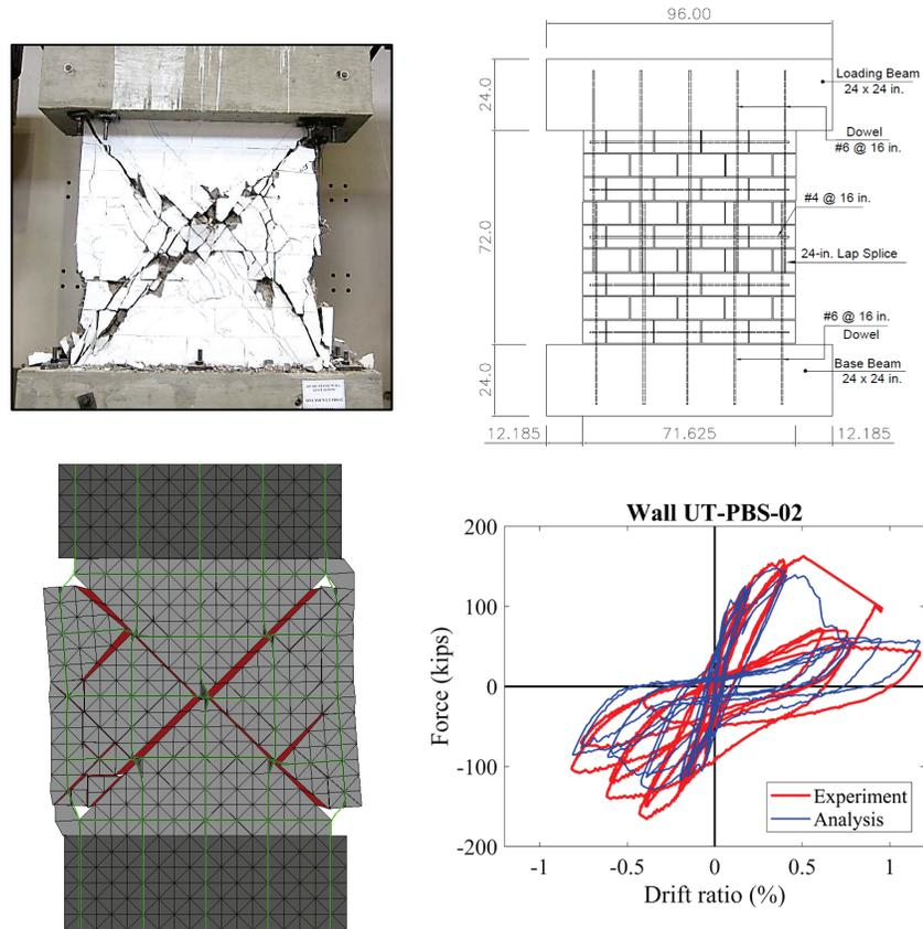
Figure 4-17 Shear-dominated wall (UT-PBS-02) tested by Ahmadi (2012).
