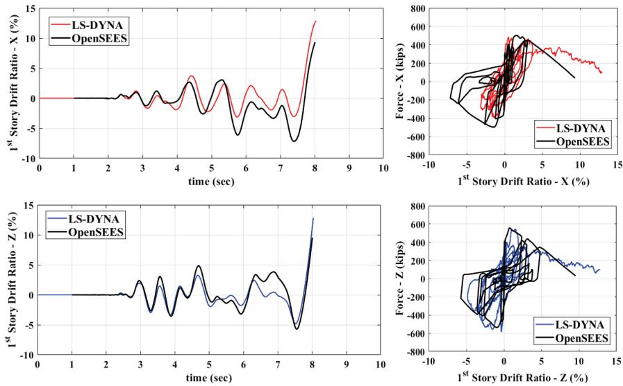
Figure B-14 Comparison of response histories for the first story: COM2 — Motion 1 ( $2 \times MCE_R$ ).
