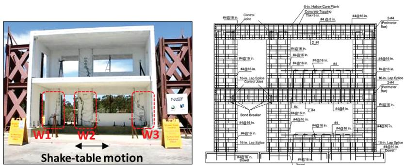
Test configuration and reinforcement details
