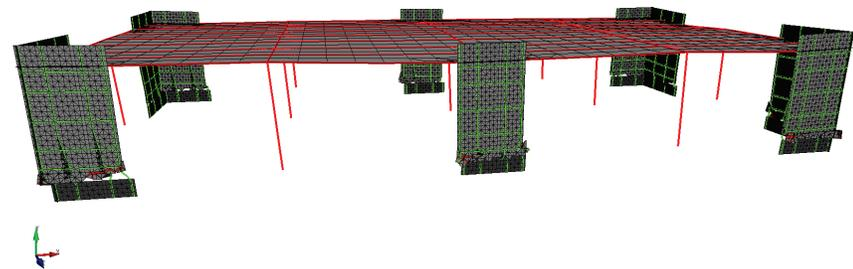
Figure B-2 Deformed meshes from refined model: COM1 (LS-DYNA) – Motion 2 ( $2.7 \times MCE_R$ ).
