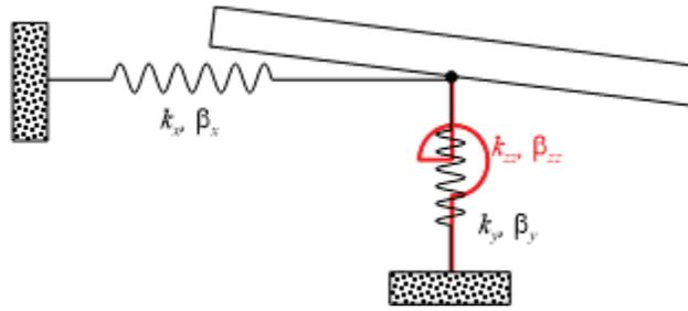
Figure C-2 Translational and rotational springs and dampers.
