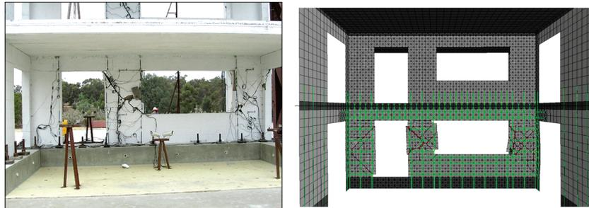
Damage in structure and model after the sequence of motions (deformations magnified by 3)
