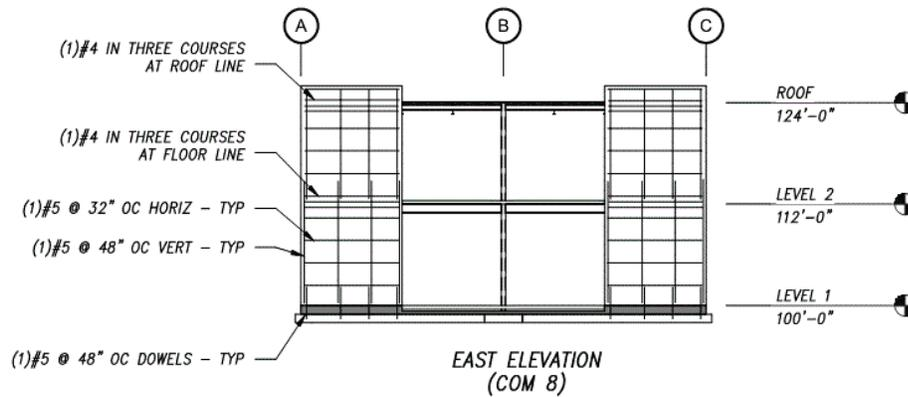
Figure A-20 Two-story commercial building East elevation: COM8.
