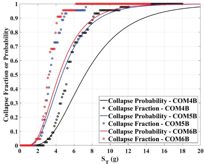
Figure 5-5 Collapse rates from IDA data and collapse fragility curves derived for very high-seismic baseline models.  $S_T$  for the collapse fraction data has been scaled by 1.2, whereas that for the collapse probability curve has been scaled by  $1.2 \times SSF$ .
