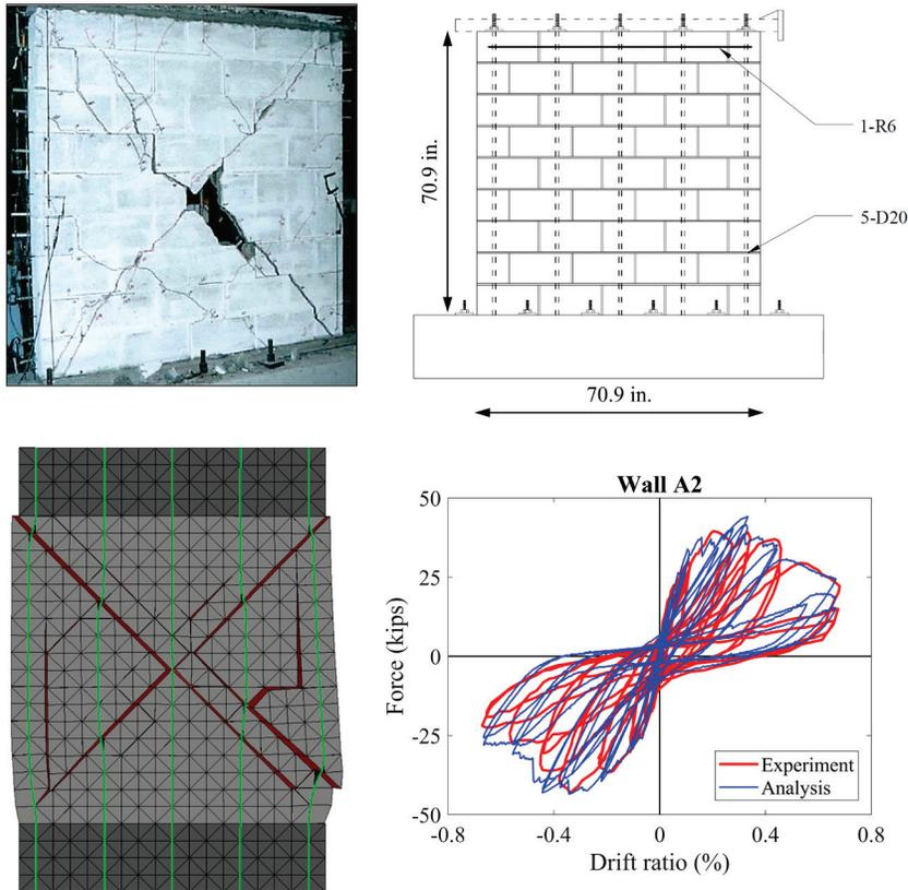
Figure 4-16 Shear-dominated wall tested by Voon and Ingham (2006).
