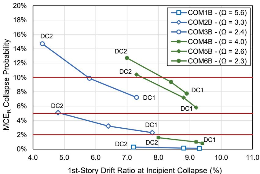
Figure 6-3  $MCE_R$  collapse probability as a function of first-story drift ratio at incipient collapse of archetype models with varying amounts of post-capping displacement capacity, and benchmark (BM) values of  $MCE_R$  collapse probability and the  $MCE_R$  collapse-safety objective of ASCE/SEI 7-10. Archetype model overstrength ( $\Omega$ ) is shown in the legend.
