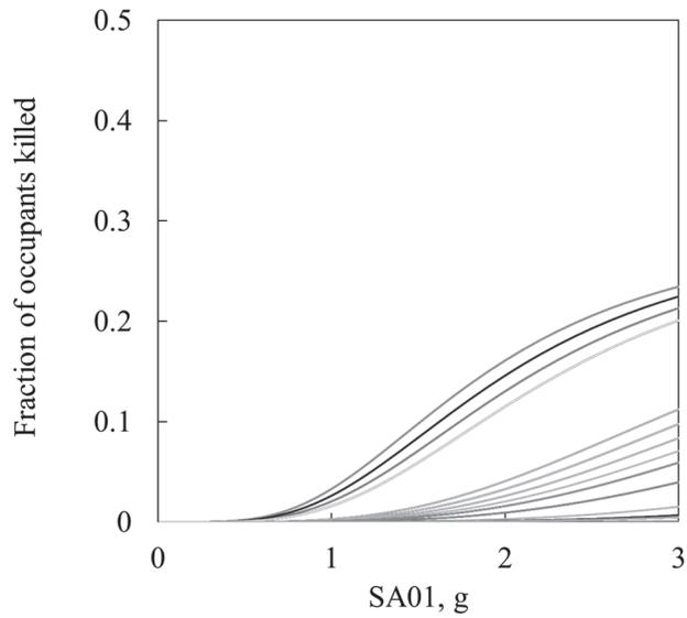
Figure H-2 Vulnerability functions for complex masonry typology, medium-resolution data.
