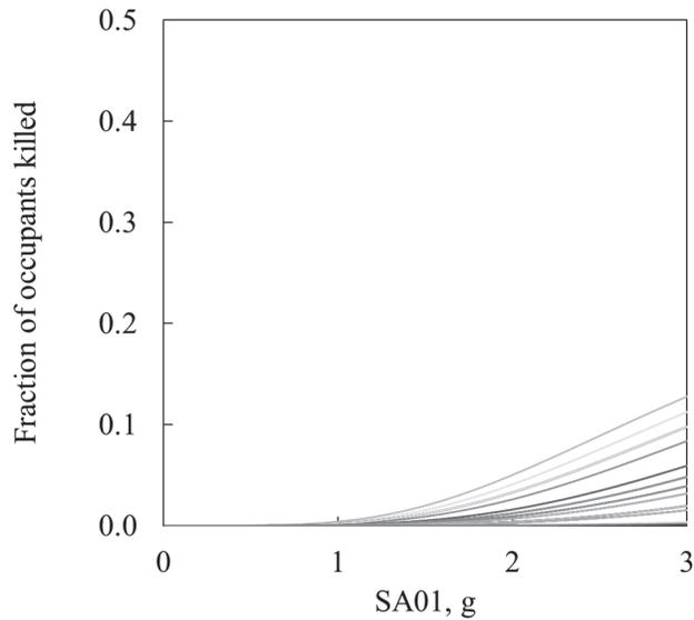
Figure H-4 Vulnerability functions for CMCF typology, medium-resolution data.
