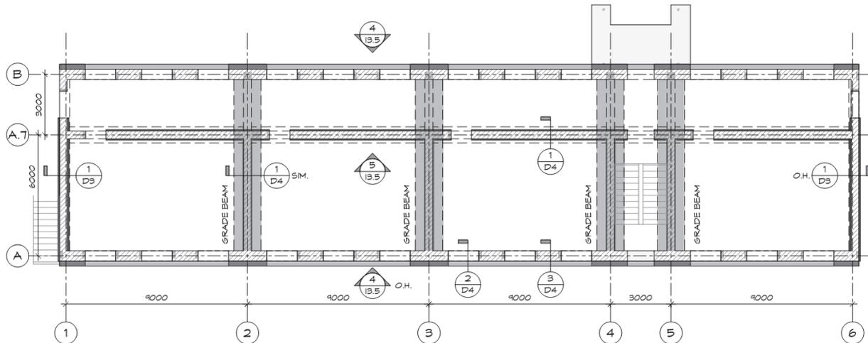
Figure 5-19 Transverse grade beams added in CM Increment 3.
