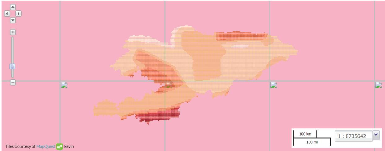
Figure 6-1 Probabilistic seismic hazard assessment map of the Kyrgyz Republic in terms of spectral acceleration expressed as fractions of g (gravit. acceleration) for a probability of exceedance of 10% over 50 years for bedrock conditions ( $V_s^{30} = 760$  m/s) (from <http://geonode.mes.kg/>, last accessed February 20, 2019).
