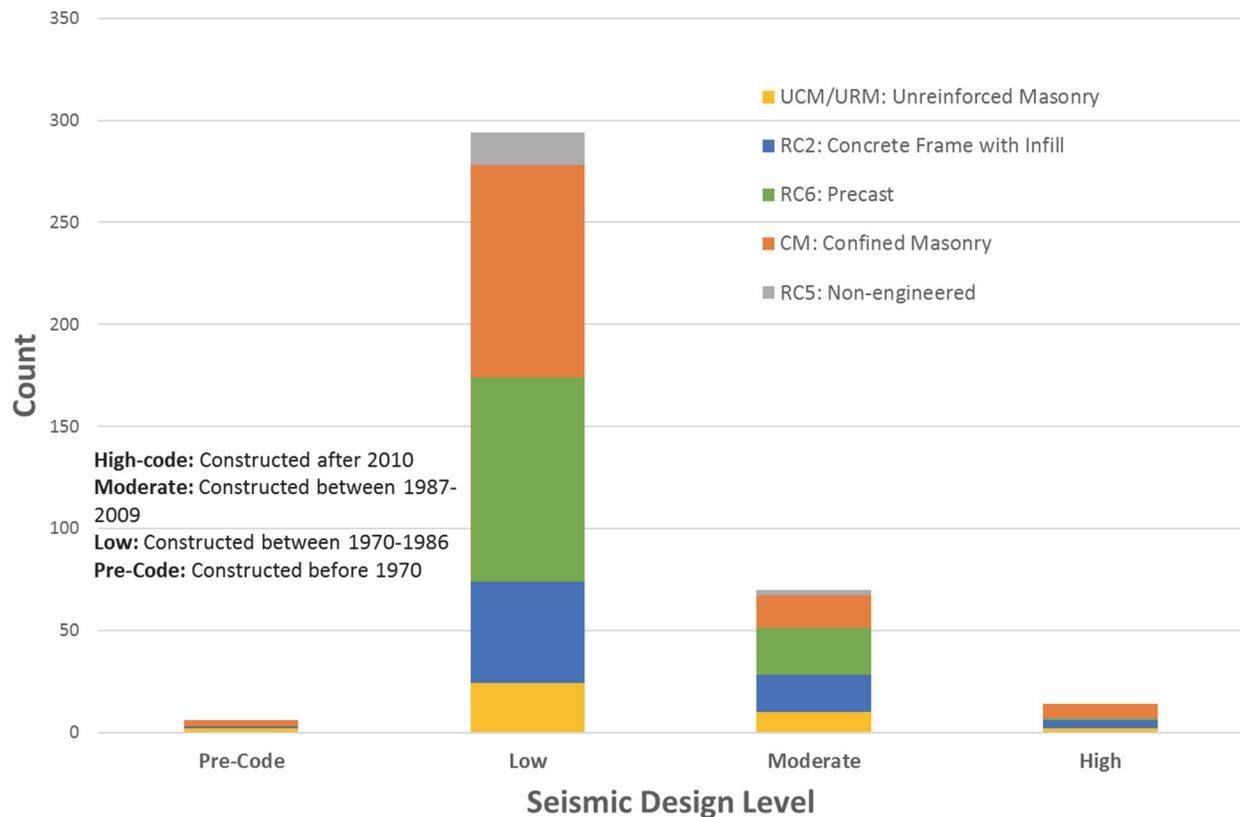
Figure 3-2 Distribution of seismic design level by school block.
