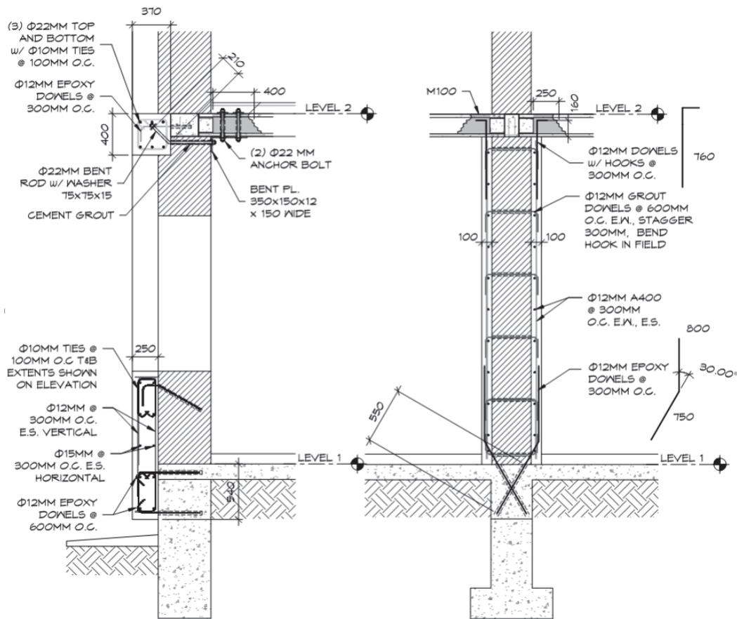
Figure 5-18 Detail of finger piers in CM Increment 2.
