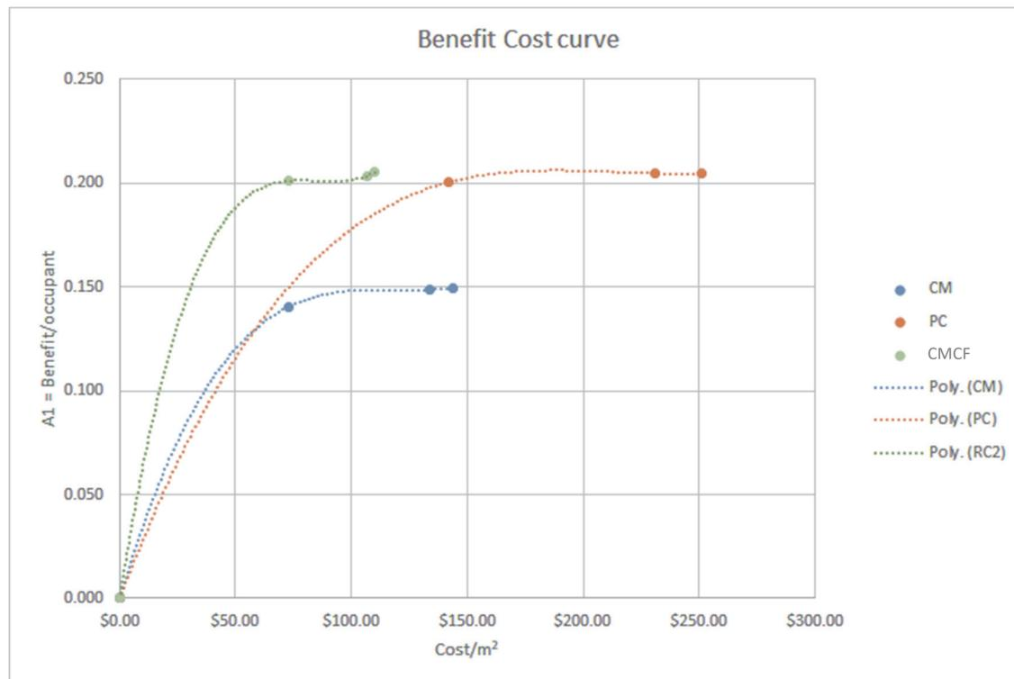
Figure 7-4 Fitted curves demonstrating the relationship between the safety/benefits index and cost for seismic retrofit.
