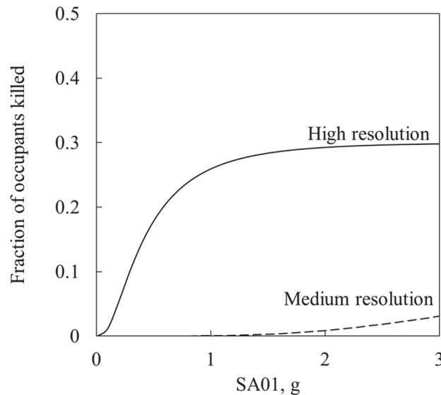
Figure H-5 Vulnerability functions for CMCF typology with medium- and high-resolution data. The medium-resolution curve represents the equally weighted average of all buildings in the group. (No buildings were mapped to CMCF from low-resolution data.)
