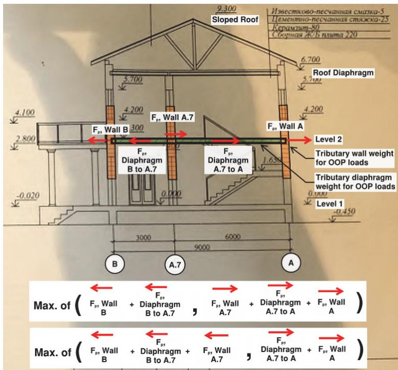
Figure 5-12 Anchorage demands for out-of-plane wall evaluations.
