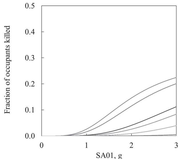
Figure H-1 Vulnerability functions for complex masonry typology, low-resolution data.
