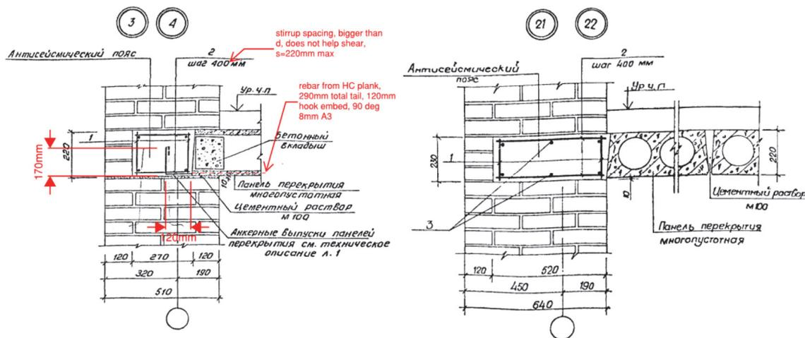
Figure 5-24 Anchorage of the structural walls.
