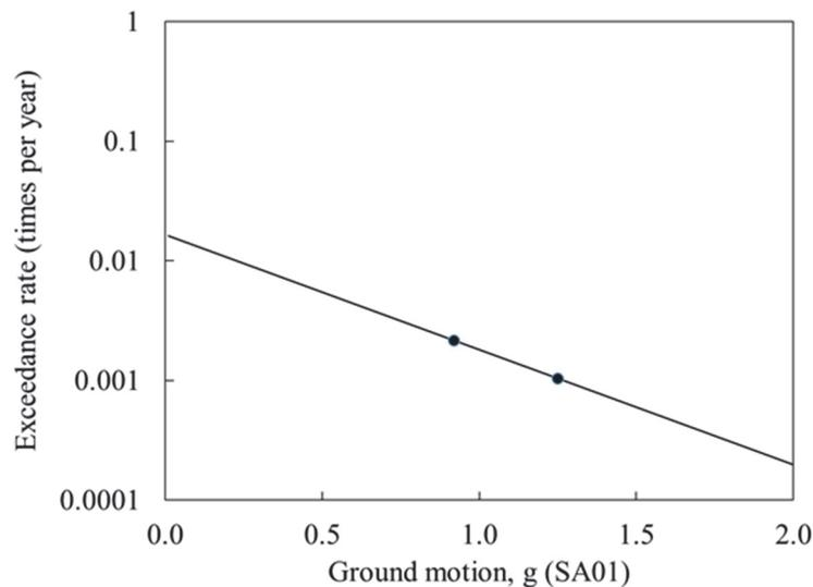
Figure 6-3 Seismic hazard curve developed from two spectral acceleration values acquired from Geonode for a given school site.
