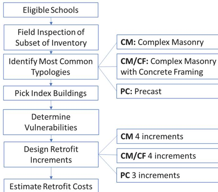
Figure 1-3 Flowchart depicting the steps of the methodology towards developing retrofit increments.
