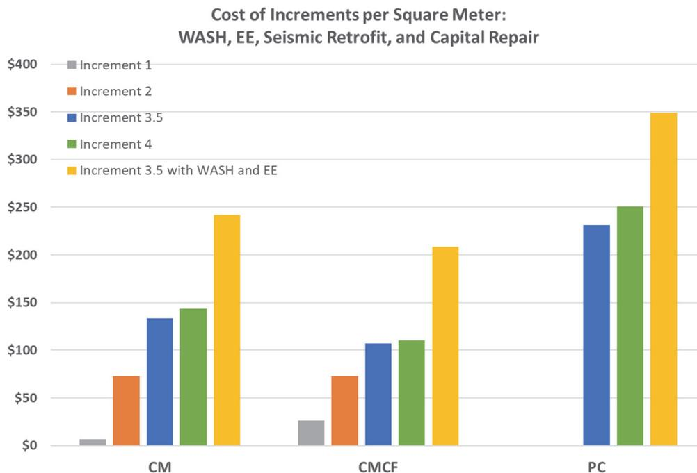
Figure 7-2 WASH, EE, seismic retrofit, and capital repair cost estimate per square meter for three typologies at retrofit increment levels.
