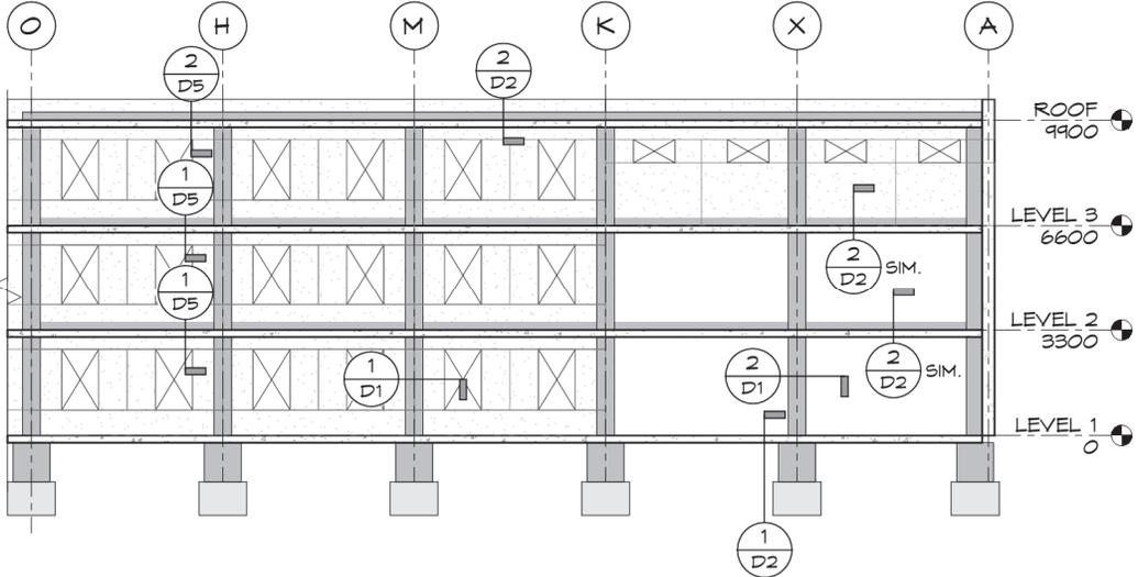
Figure 5-44 Elevation showing jacketed columns in PC Increment 2.
