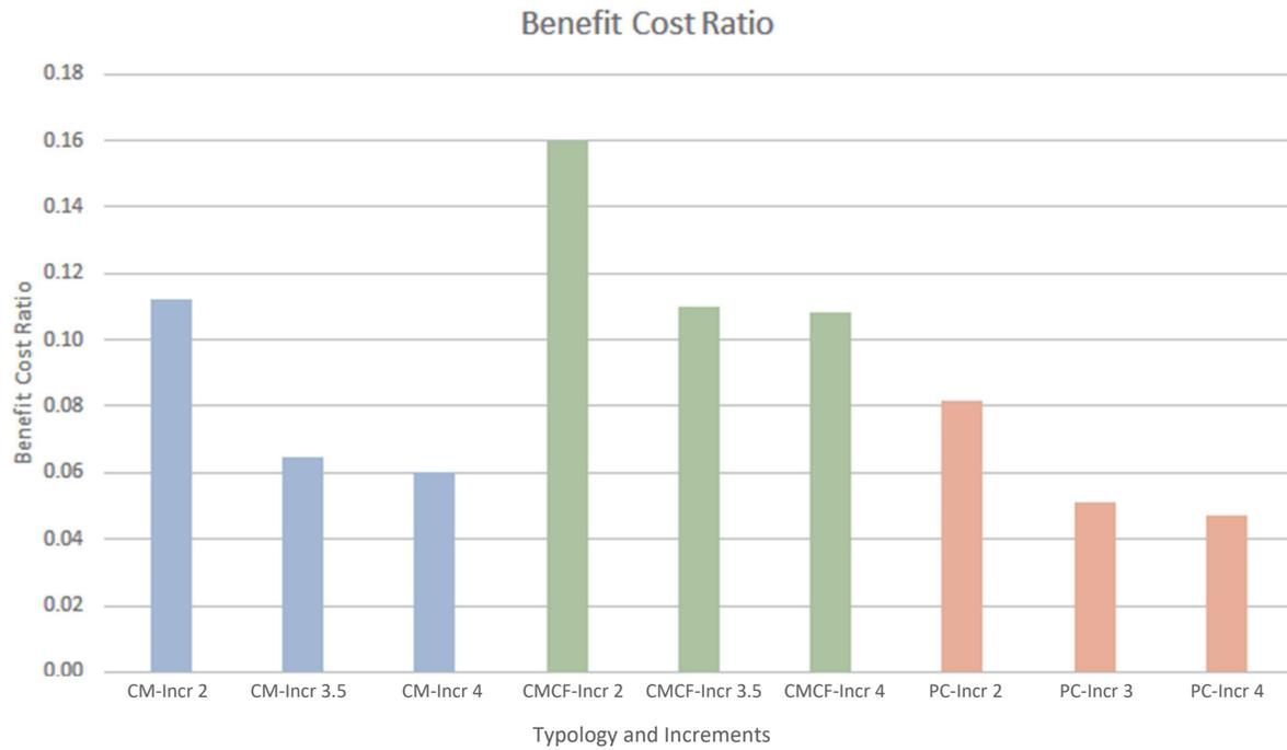
Figure 7-3 Comparison of benefit-cost ratio for retrofit increments of identical buildings constructed with different typologies.
