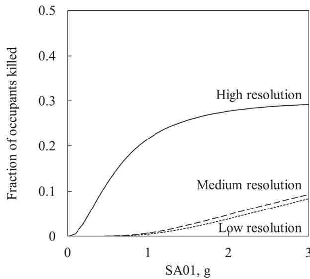
Figure H-3 Vulnerability functions for complex masonry typology, low-, medium-, and high-resolution data. Low- and medium-resolution curves reflect the equally weighted average of all buildings in the group.
