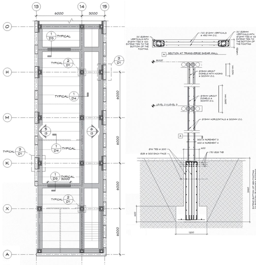
Figure 5-47 Transverse walls and foundation added for PC Increment 3.
