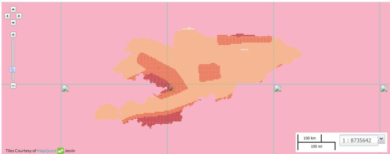
Figure 6-2 Probabilistic seismic hazard assessment map of the Kyrgyz Republic in terms of spectral acceleration expressed as fractions of g (gravit. acceleration) for a probability of exceedance of 5% over 50 years for bedrock conditions ( $V_s^{30} = 760$  m/s) (from <http://geonode.mes.kg/> last accessed February 20, 2019).
